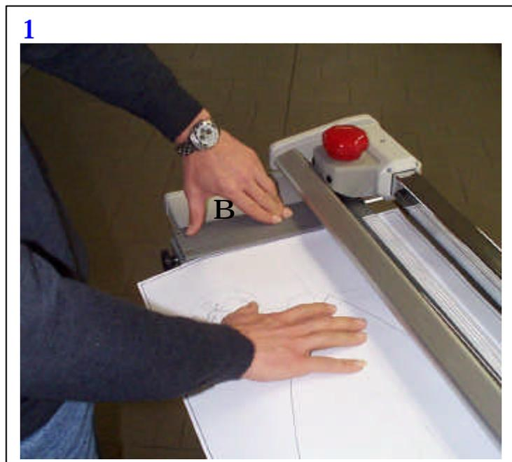
Execute the cut moving the carriage carry blade from right to left or vice versa **2**.
