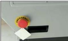
Emergency stop is which is used in emergent situation.It should be pressed after dealing with emergency.Then press the PESET button to get into functional
