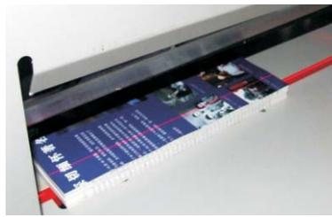
Turn the protective switch to ON position. Screen display will be light and the indicative line light on the machine will be bright. The machine can be operated after background is calibrated automatically.
