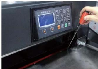
Note: When knife shim is being changed, the blade itself also needs to be adjusted. If the blade cuts too deep, the knife will be damaged easily, and the blade also will abrade rapidly.
