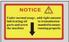
Under normal usage,please add right amount lubricating oil to transmission parts and screw mandrel to ensure the machine running properly.
