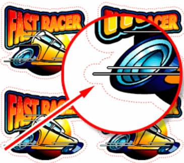
When your design is successfully imported into EasySIGN, you should then select the line or lines that you want to cut on your plotter. After selecting them, use the command "Edit, Convert to, Line type, Print&cut line". The lines that will be cut are now shown in a dotted red line. Copy the design as you like.
