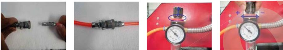
1. Connect the heat press with air compressor or air sources.
