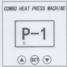
Once the SET button is pressed, the foregoing picture will emerge, it will shows P-1 it indicates setting temperature, then the parameters can be adjusted by pressing ▼ or ▲.
