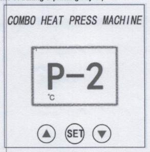
Press the "SET" button second time, the foregoing picture will emerge. It shows P-2,it indicates setting time, then the parameters can be adjusted by pressing ▼ or ▲.
