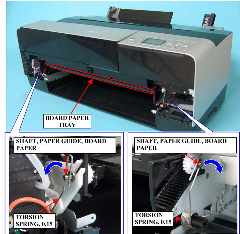
Figure 4-62. Removing the TORSION SPRING, 0.15
