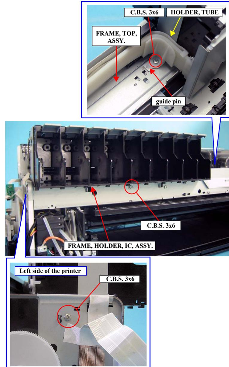
Figure 4-82. Removing the screws from the FRAME, HOLDER, IC, ASSY.
