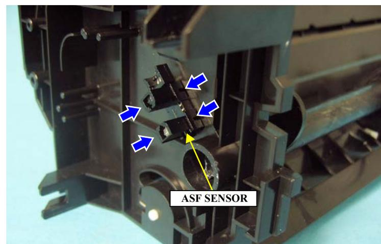
Figure 4-155. Removing the ASF SENSOR
