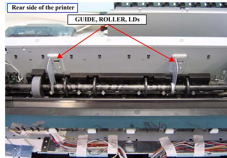
Figure 4-148. Removing the GUIDE, ROLLER, LDs
