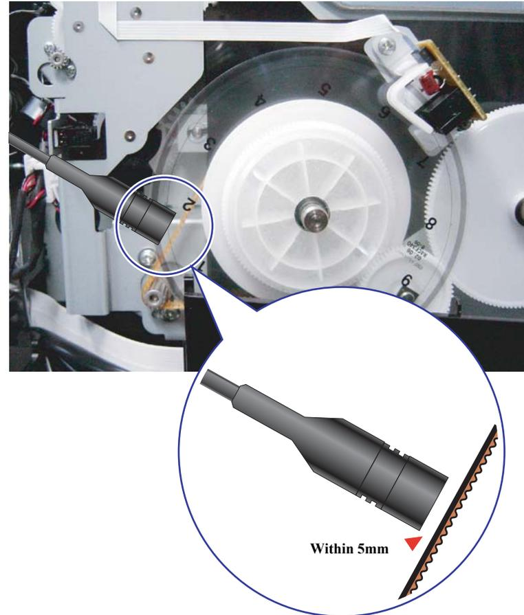
Figure 5-4. Tension Measurement
