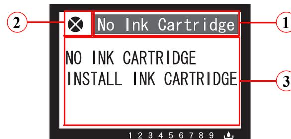
Figure 1-9. Panel Display (Error indication)
