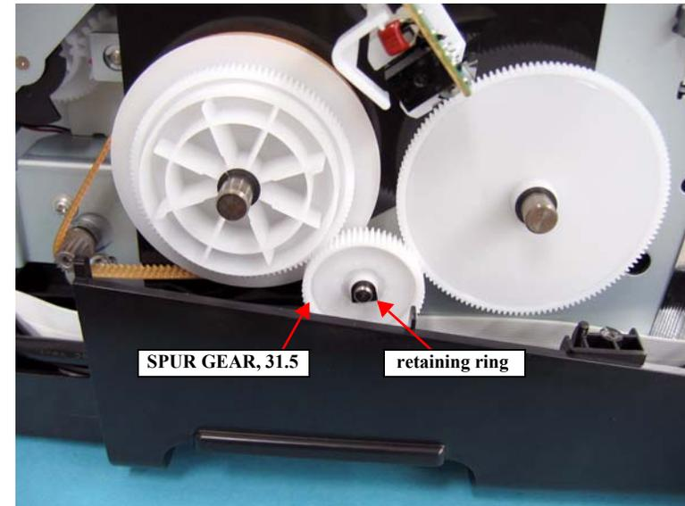
Figure 4-127. Removing the SUPUR GEAR, 31.5 (1)
