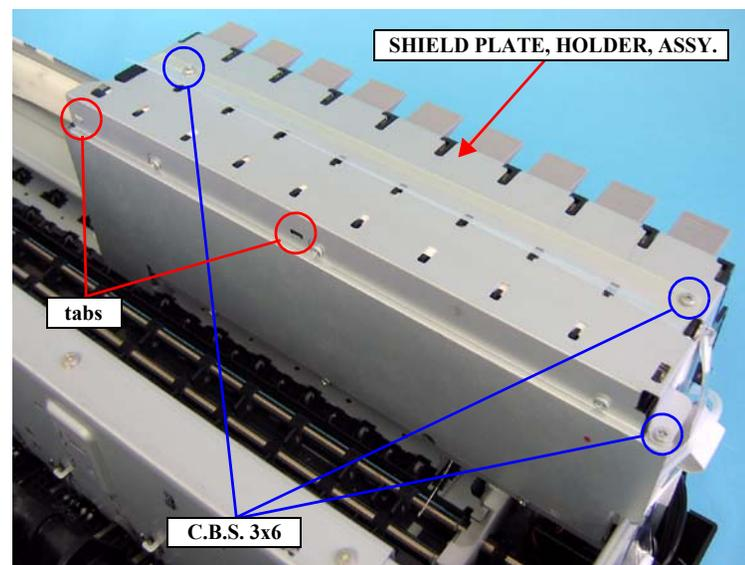
Figure 4-80. Removing the SHIELD PLATE, HOLDER, ASSY.
