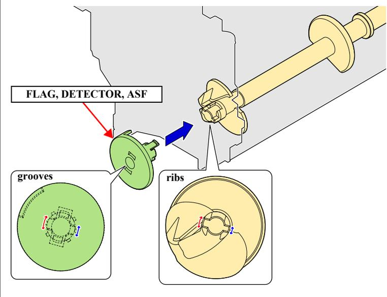
4. Disengage the four tabs of the ASF SENSOR, and remove the ASF SENSOR.
