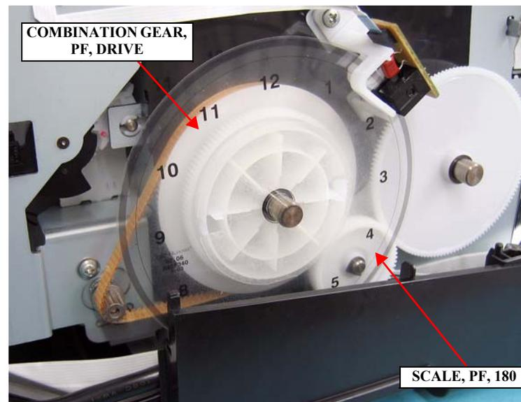
Figure 4-126. Removing the SCALE, PF, 180
