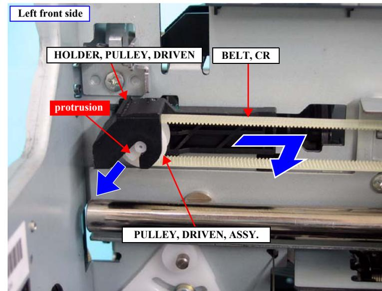
Figure 4-153. Removing the PULLEY, DRIVEN, ASSY.
