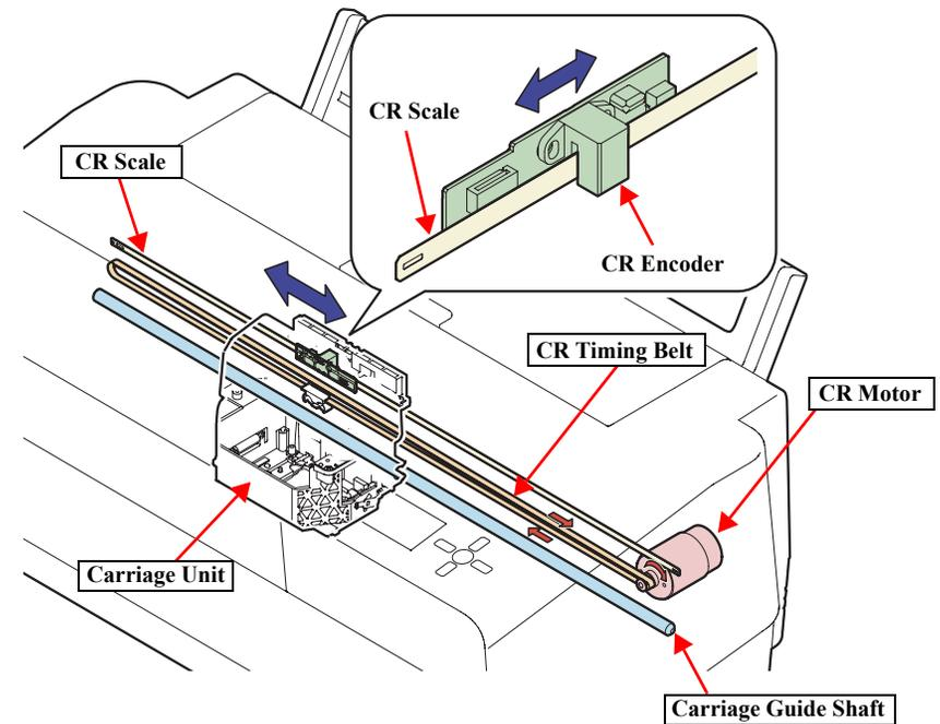
Figure 2-15. Carriage Movement Mechanism
