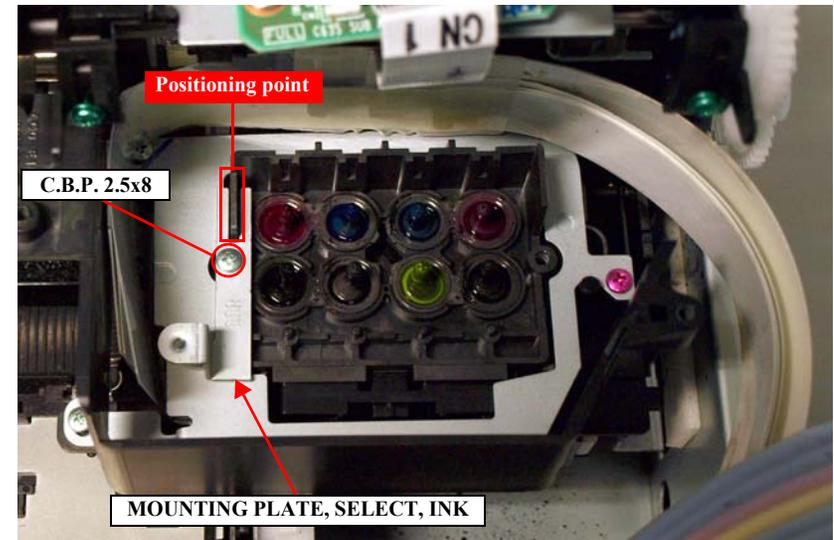
Figure 4-108. Installing the MOUNTING PLATE, SELECT, INK
