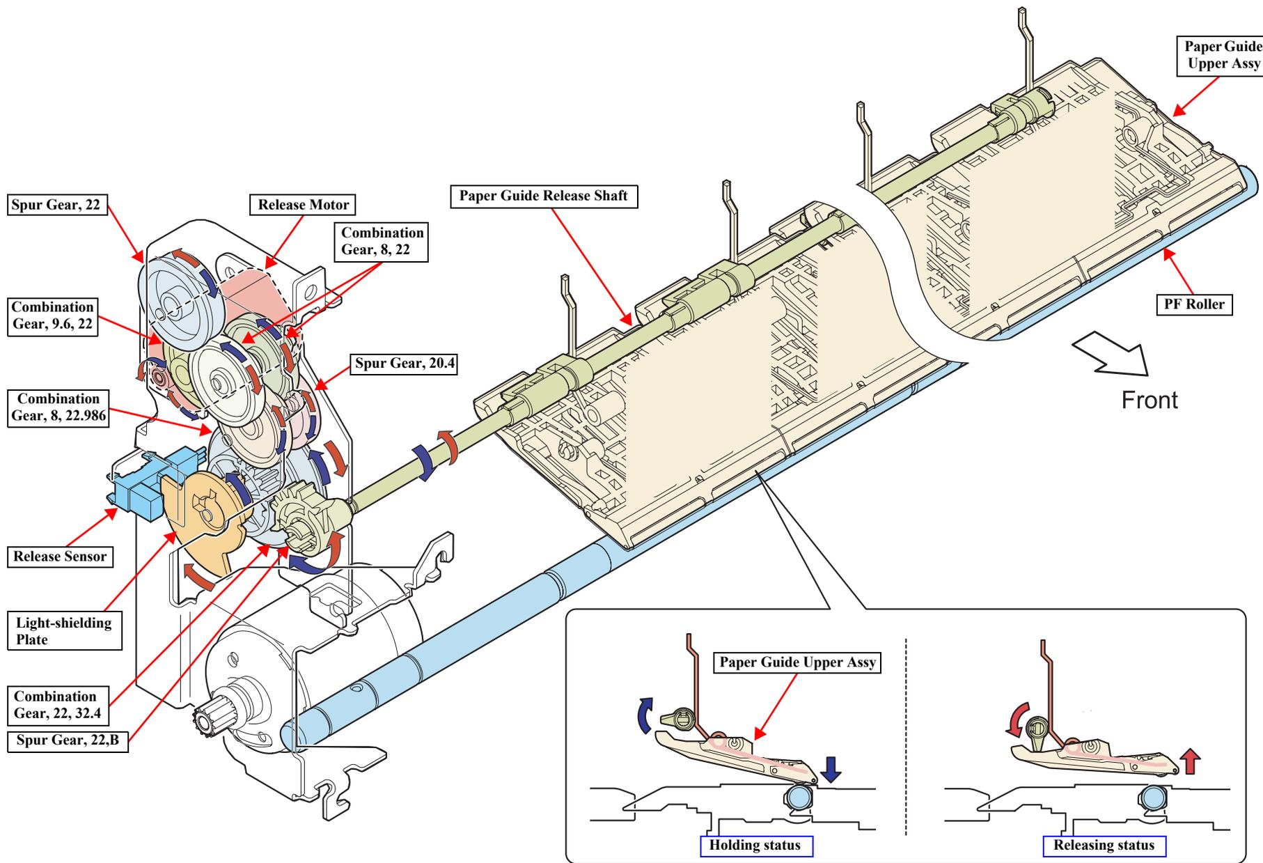
Figure 2-28. Release Mechanism
