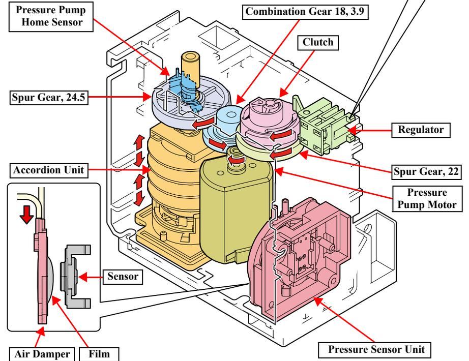
Figure 2-8. Pressure Pump Unit
