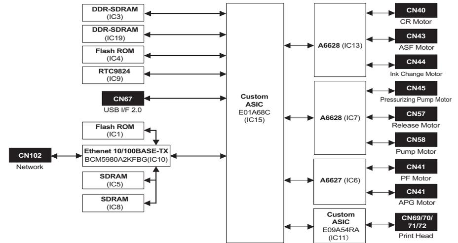
Figure 2-33. C635/CA61 MAIN Board Block Diagram
