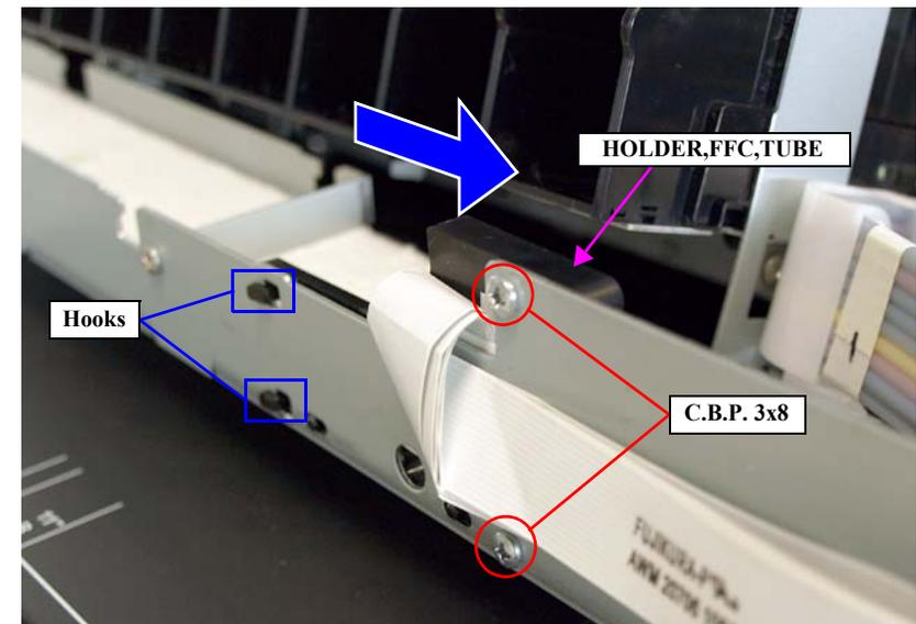
Figure 4-101. Removing the HOLDER,FFC,TUBE
