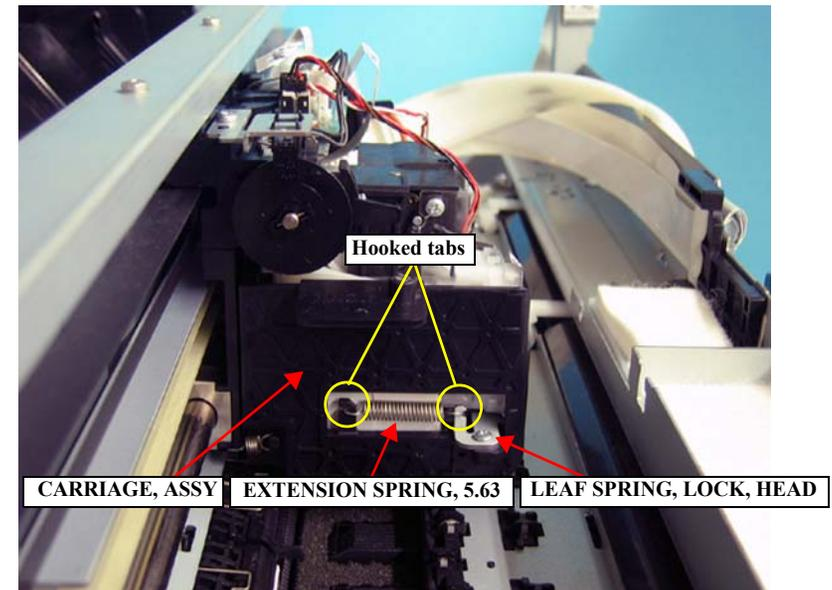
Figure 4-109. Attaching the EXTENSION SPRING, 5.63
