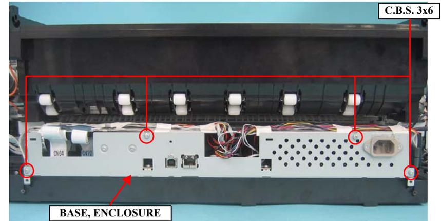
Figure 4-27. Removing the screws from the BASE, ENCLOSURE
