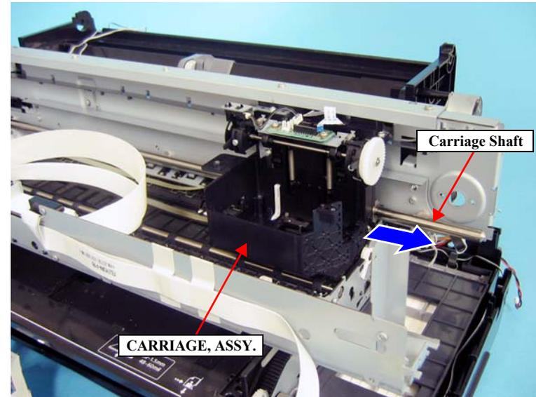
Figure 4-139. Removing the CARRIAGE, ASSY.
