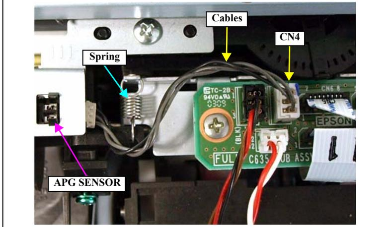
11. Secure the grounding wire to the BOARD ASSY., SUB with the screw.
