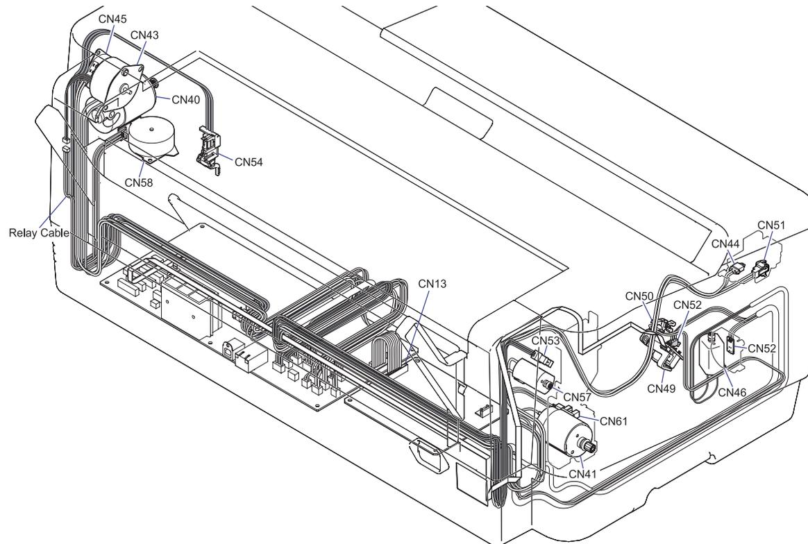
Figure 7-4. Routing Layout (3)
