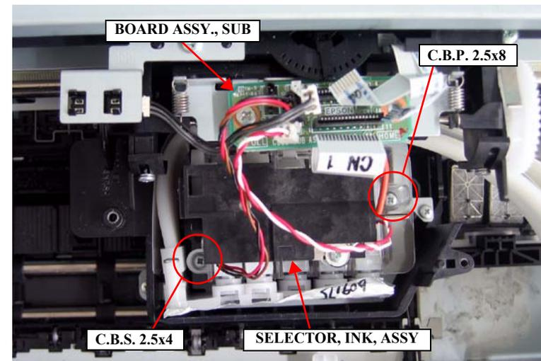
Figure 4-111. Installing the SELECTOR, INK, ASSY
