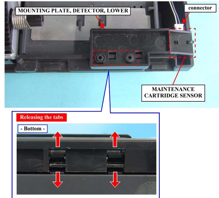
Figure 4-51. Removing the MOUNTING PLATE, DETECTOR, LOWER
