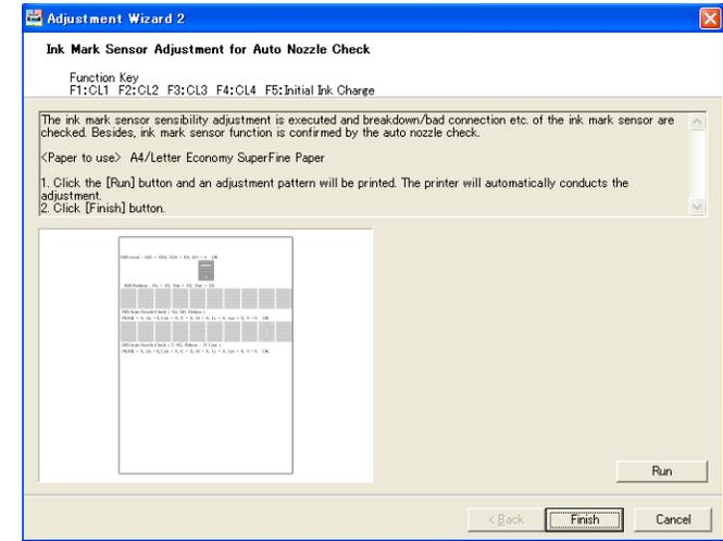
Figure 5-58. [Ink Mark Sensor Adjustment for Auto Nozzle Check] Screen
