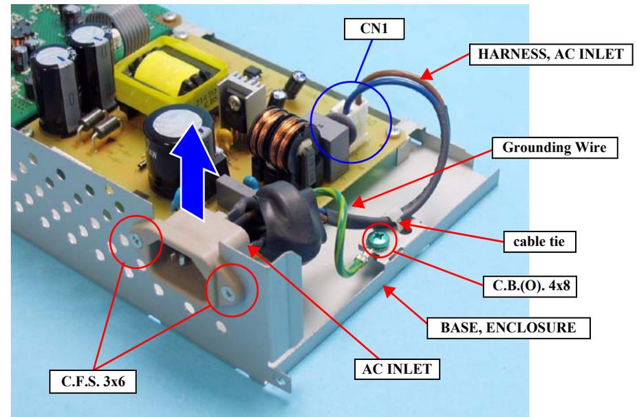
Figure 4-35. Removing the AC INLET
