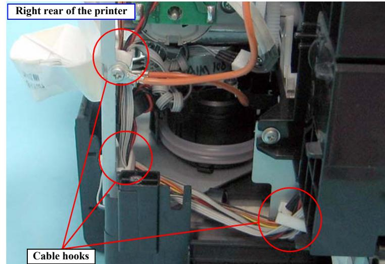
Figure 4-38. Releasing the MOTOR ASSY., APG cables (1)
