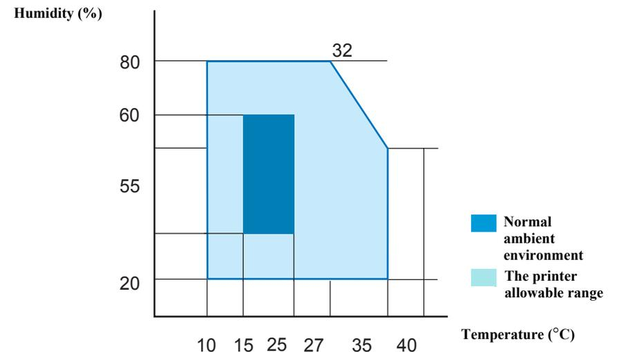
Figure 1-2. Temperature/Humidity Range
