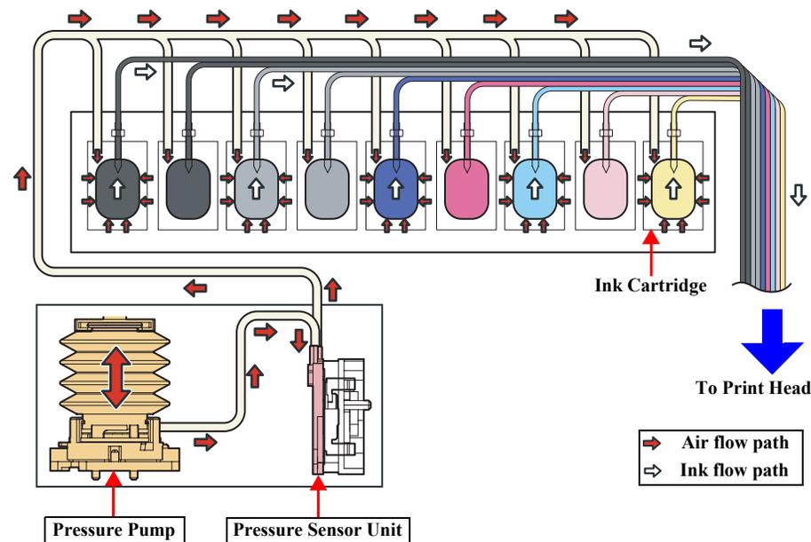
Figure 2-6. Ink Pressurizing Mechanism
