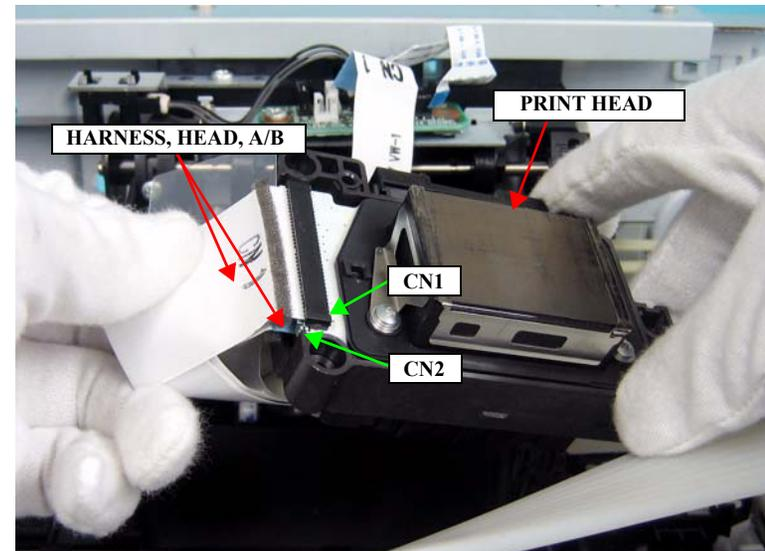
Figure 4-105. Installing the PRINT HEAD
