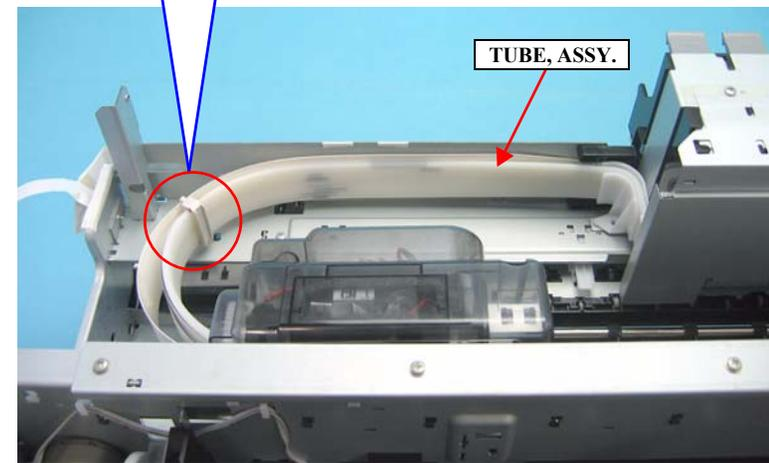
Figure 4-83. Releasing the TUBE, ASSY.
