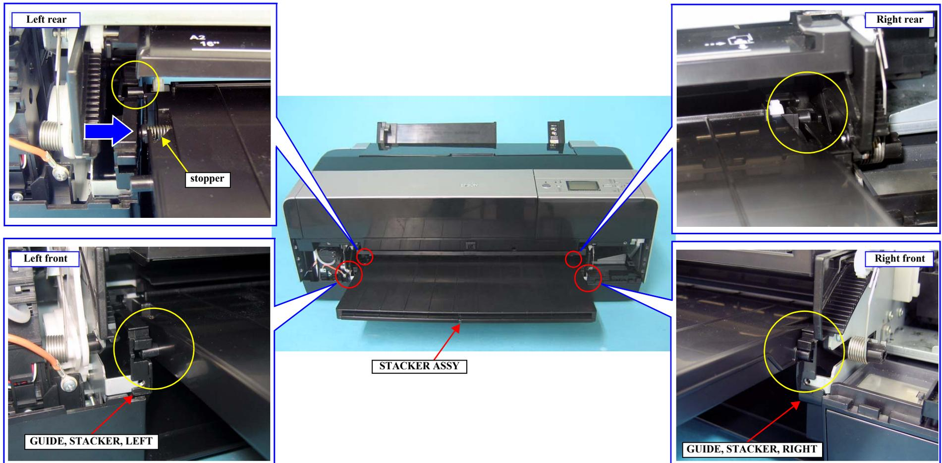
Figure 4-61. Installing the STACKER, ASSY
