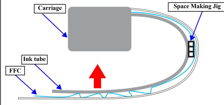
13. With the “Space Making Jig” is attached, temporarily secure the ink tube, FFC, GUIDE, TUBE, CR with acetate tape.
