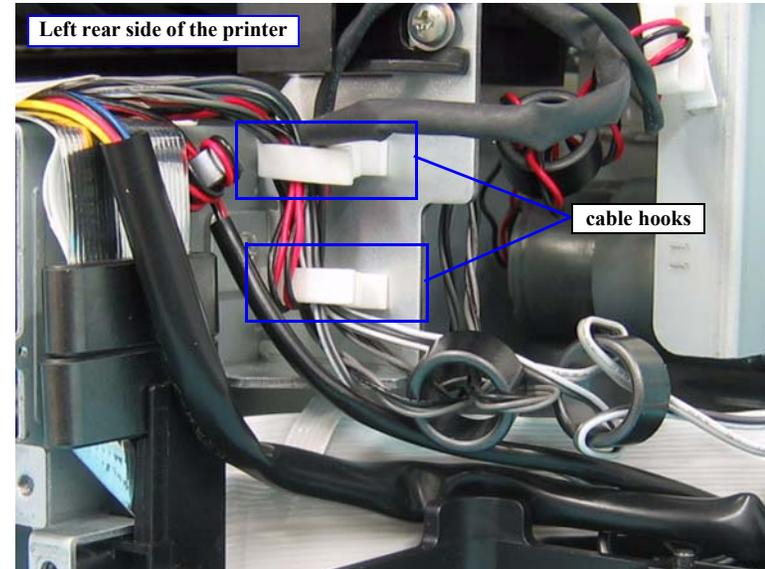
Figure 4-47. Releasing the LOCK, COVER, ASSY. Cables (1)
