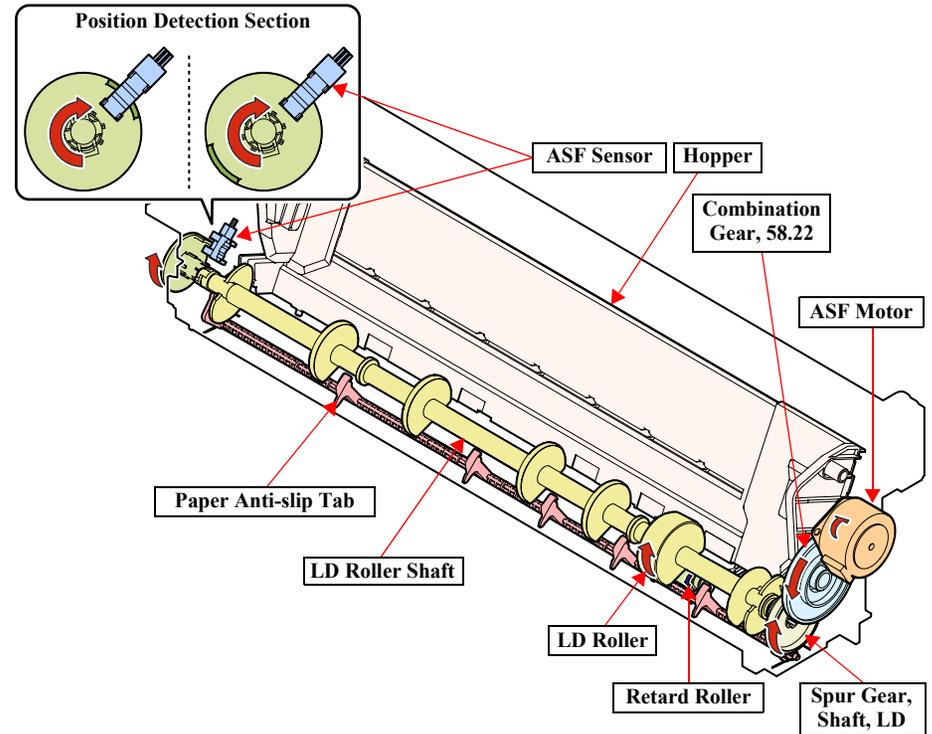
Figure 2-24. ASF Drive Mechanism
