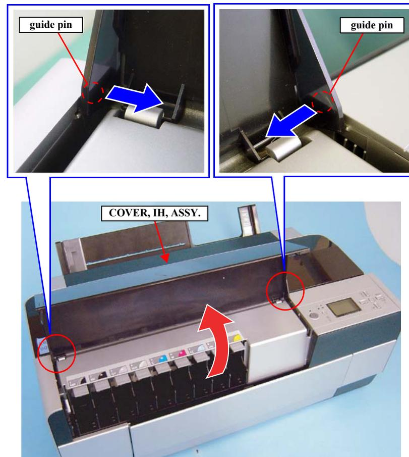
Figure 4-7. Removing the COVER, IH, ASSY.
