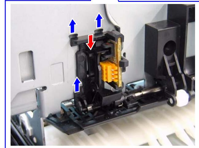
Figure 4-158. Removing the PAPER, DETECTOR, ASSY.
