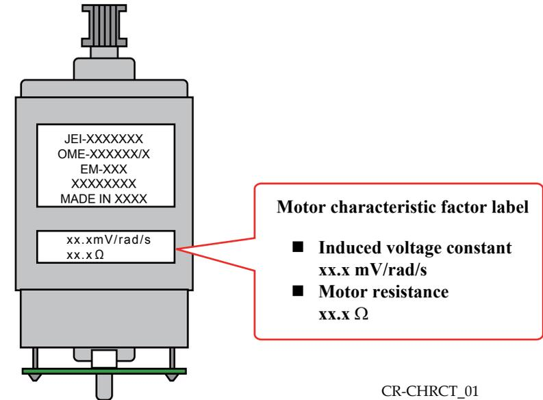
Figure 5-78. Motor Characteristic Factor Label
