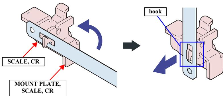
Figure 4-55. Removing the SCALE, CR (2)
