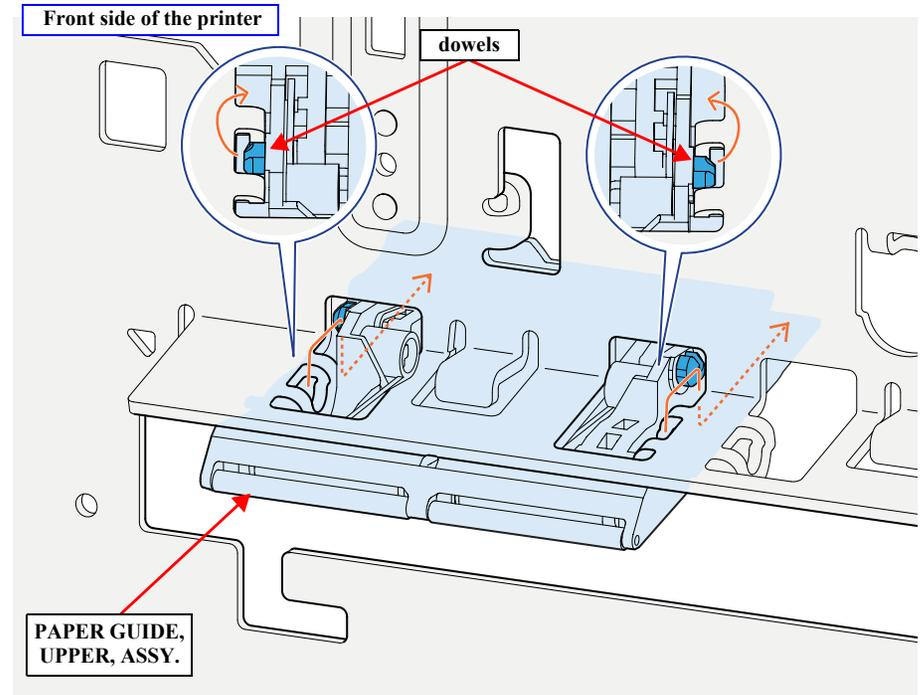
Figure 4-162. Removing the PAPER GUIDE, UPPER, ASSY.
