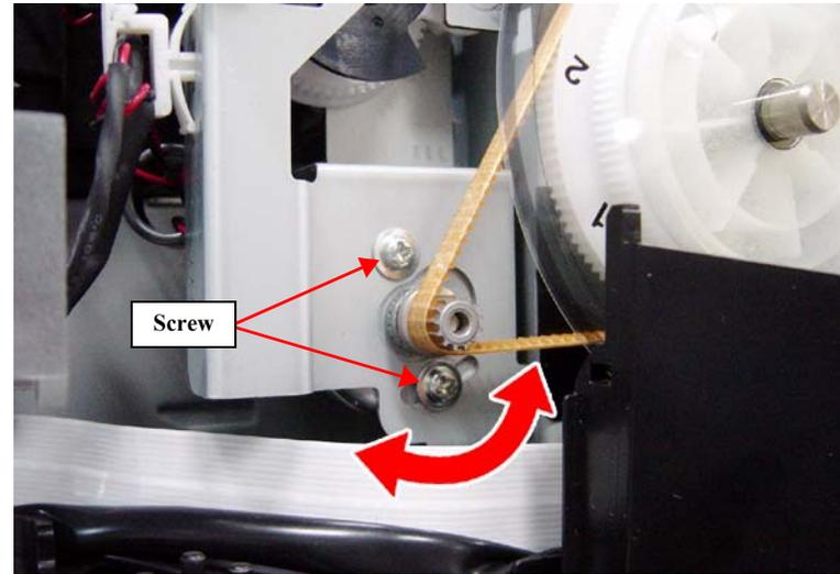
Figure 5-5. Tension Adjustment
