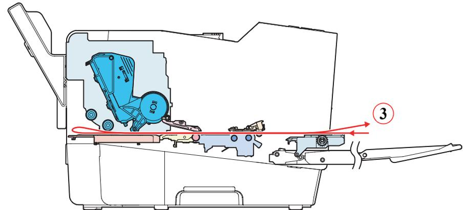
Figure 2-19. Paper Path of Front Manual Bypass
