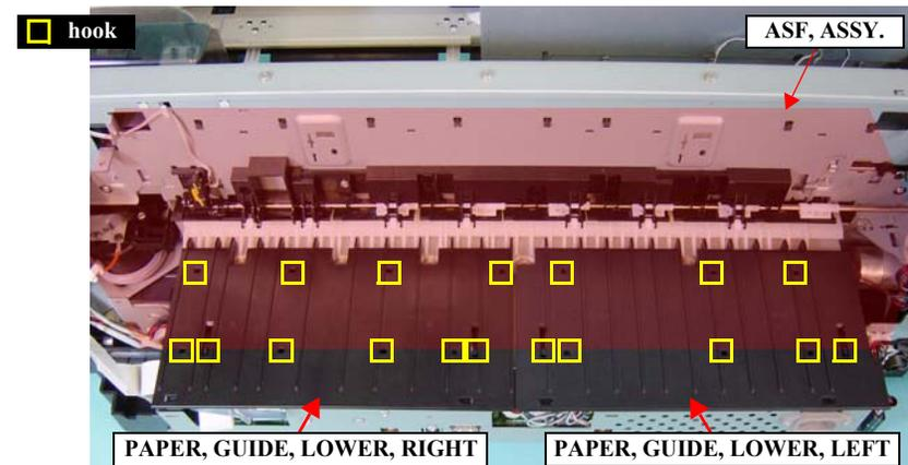
Figure 4-26. Removing the PAPER, GUIDE, LOWER, LEFT/RIGHT
