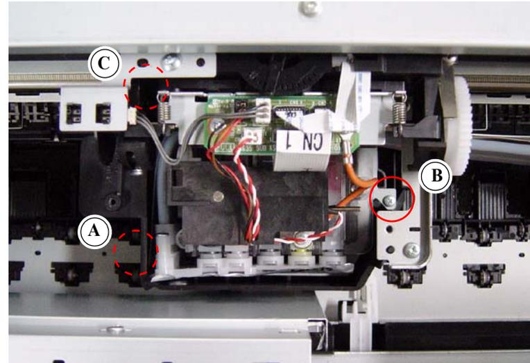
Figure 5-23. Screws Securing the [LEAF SPRING, LOCK, HEAD]
