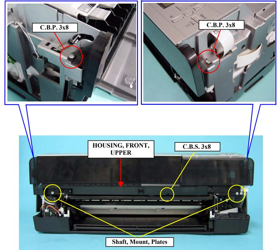
Figure 4-16. Removing the HOUSING, FRONT, UPPER
