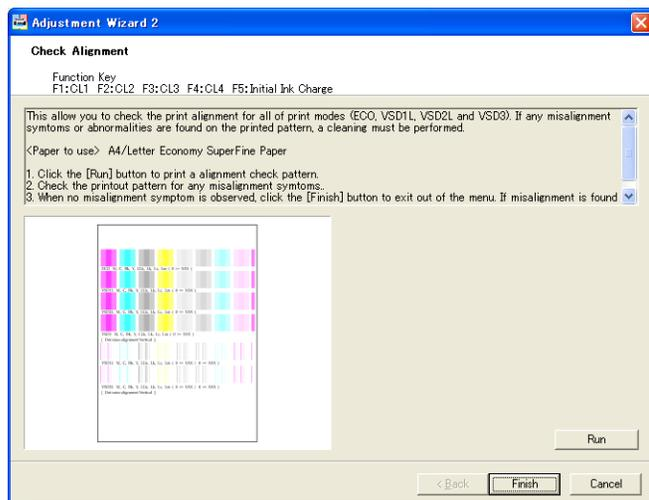
Figure 5-85. [Check Alignment] Screen
