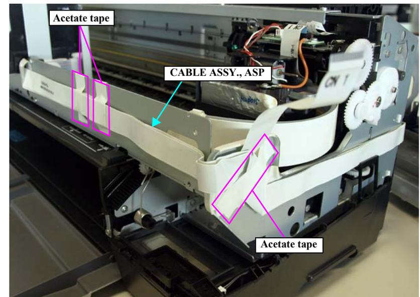
Figure 4-103. Releasing the CABLE ASSY., ASP
