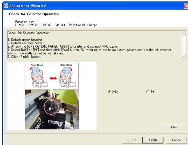
Figure 5-76. [Check Ink Selector Operation] Screen
