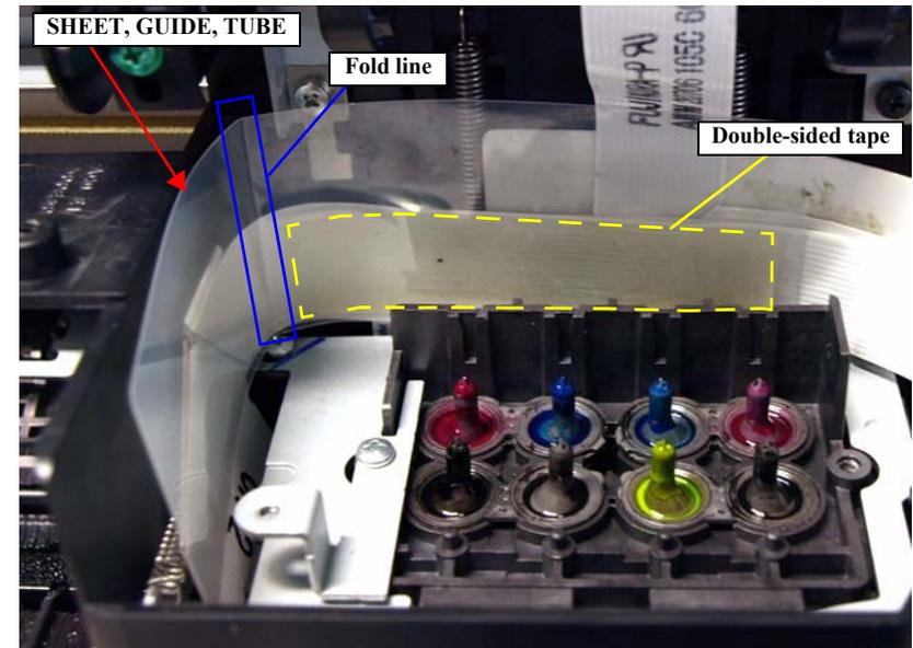
Figure 4-110. Attaching the SHEET, GUIDE, TUBE
