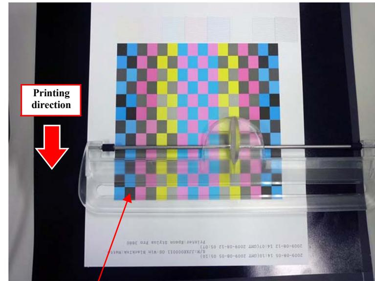
Set the scanning ruler with its slot matched with the patch.
