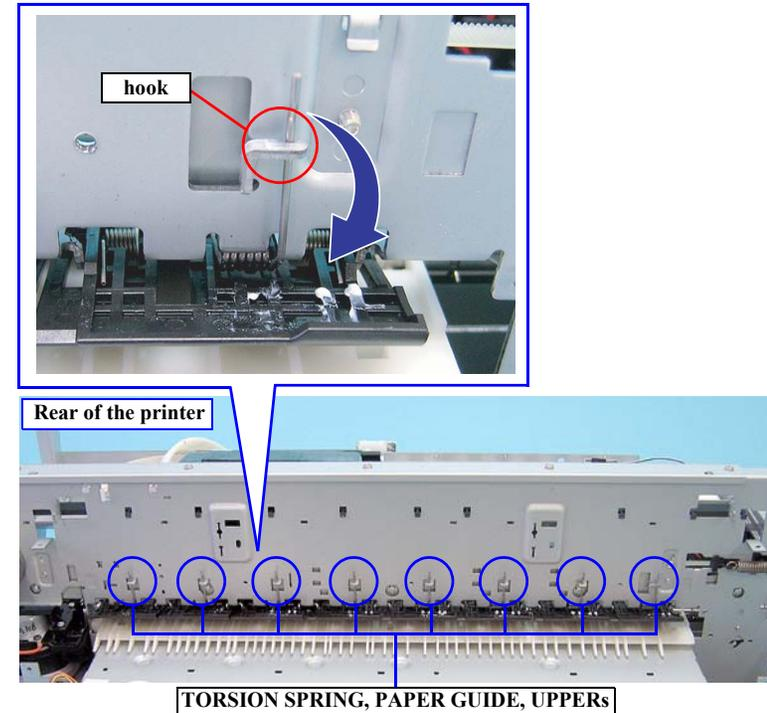
Figure 4-161. Removing the TORSION SPRING, PAPER GUIDE, UPPERS
