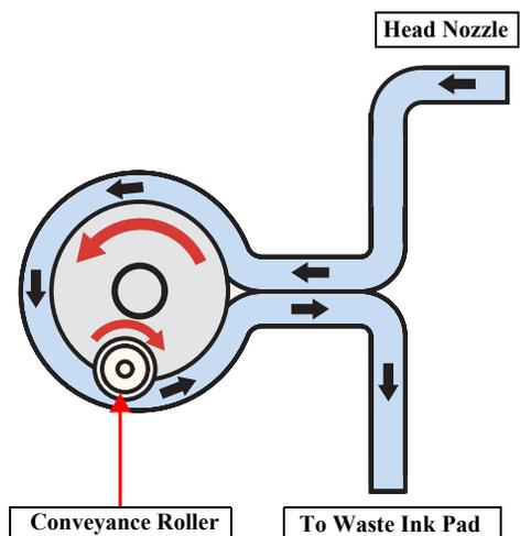
Figure 2-13. Pump Unit Mechanism
