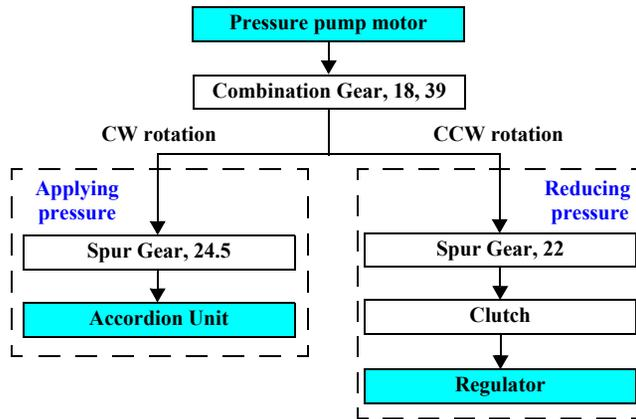
Figure 2-7. Drive Transmission Path
