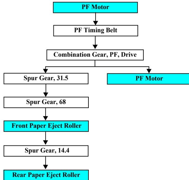
Figure 2-29. Drive Transmission Path
