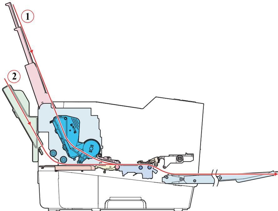
Figure 2-18. Paper Path of ASF & Rear Manual Bypass
