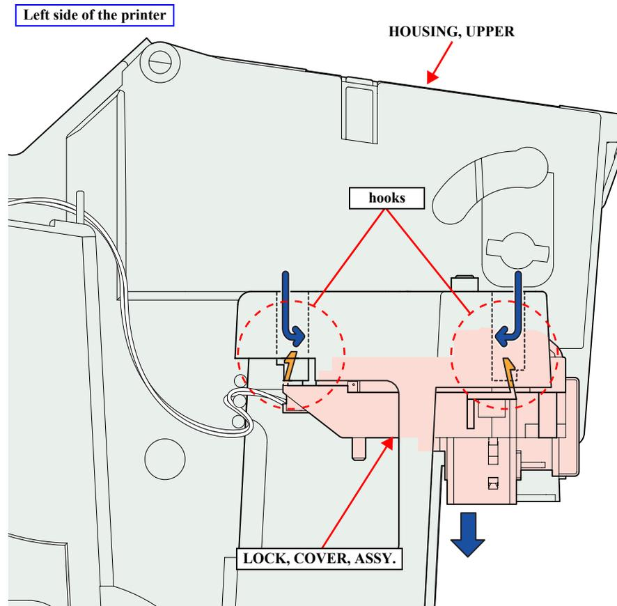
Figure 4-45. Removing the LOCK, COVER, ASSY.
