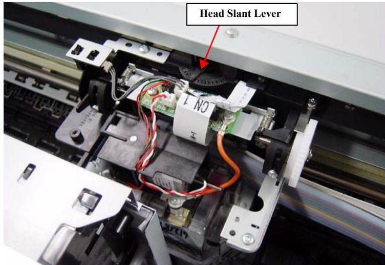
Figure 5-16. Head Slant Lever
