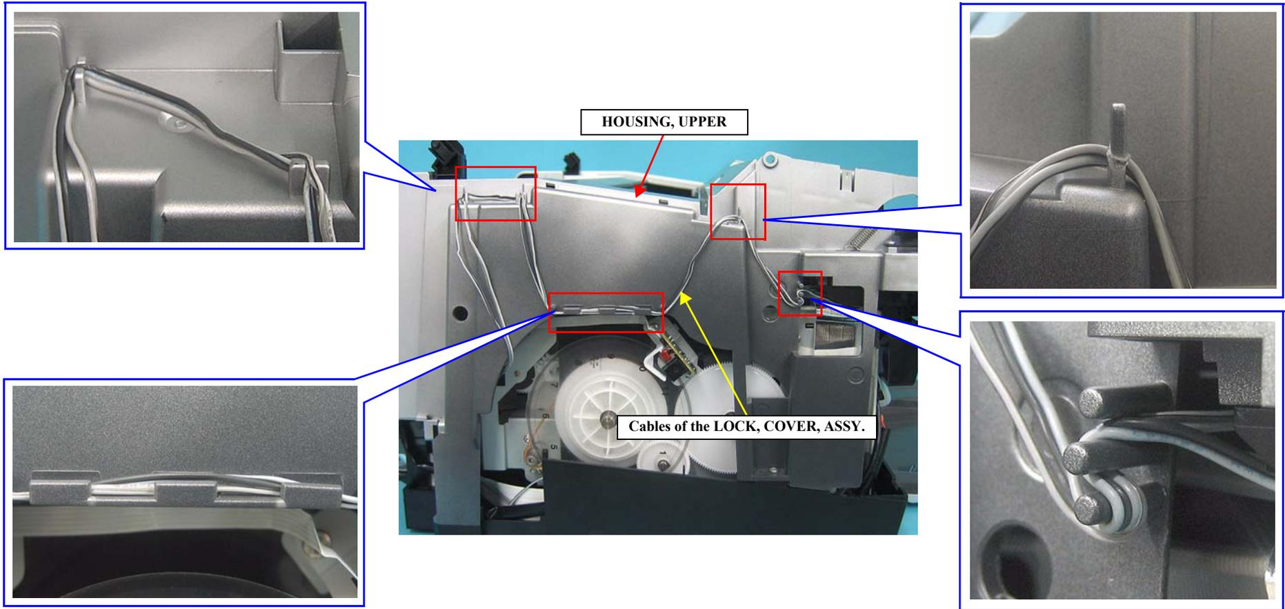
Figure 4-46. Routing the LOCK, COVER, ASSY. Cables
