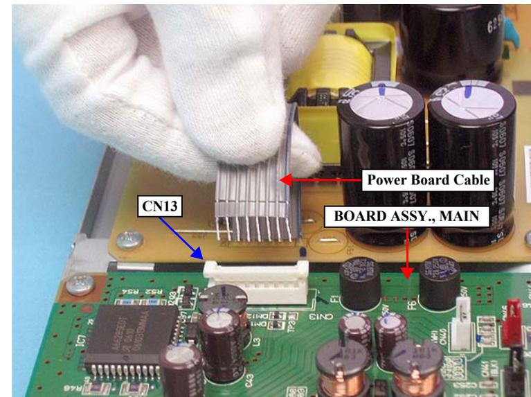
Figure 4-30. Disconnecting the Power Board Cable from CN13
