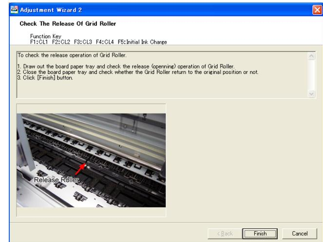
Figure 5-66. [Check the Release Of Grid Roller] Screen
