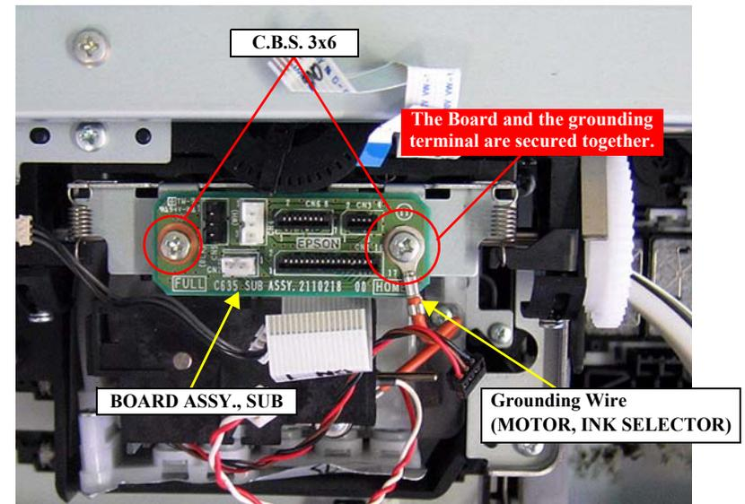
Figure 4-37. Removing the BOARD ASSY., SUB
