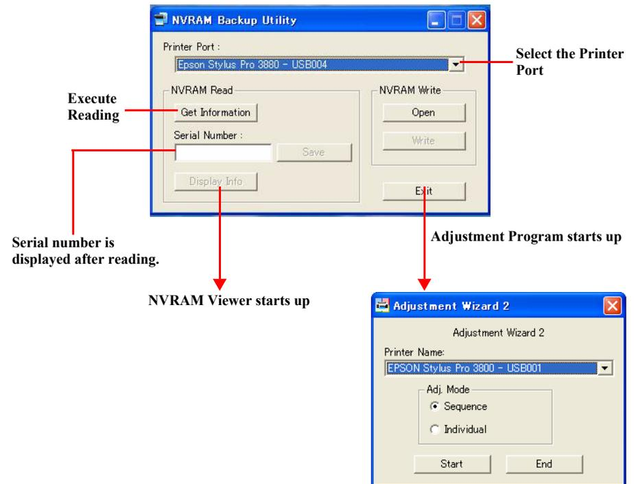
Figure 5-30. NVRAM Back Up Utility Screen Transition
