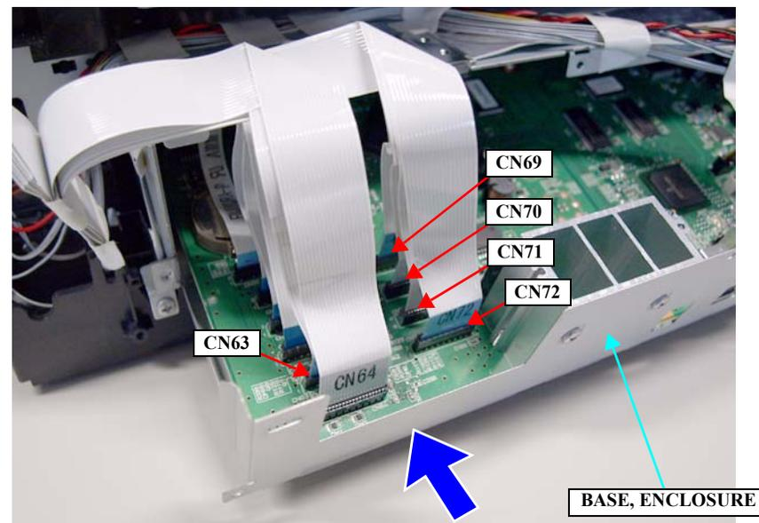
Figure 4-124. Connecting the Cables
