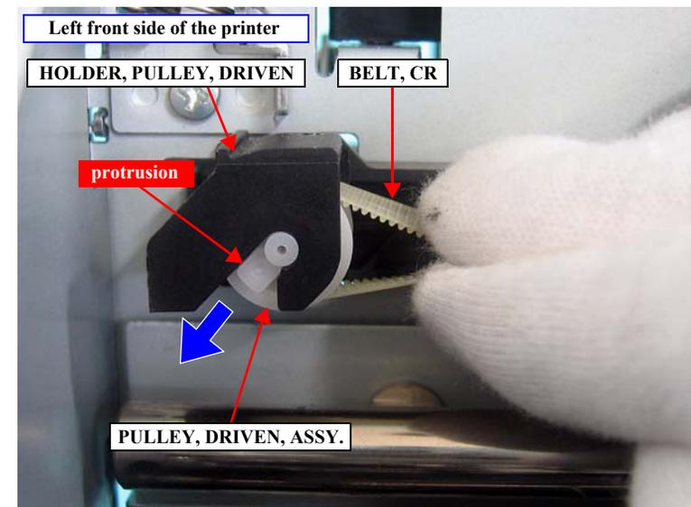
Figure 4-136. Removing the PULLEY, DRIVEN, ASSY.
