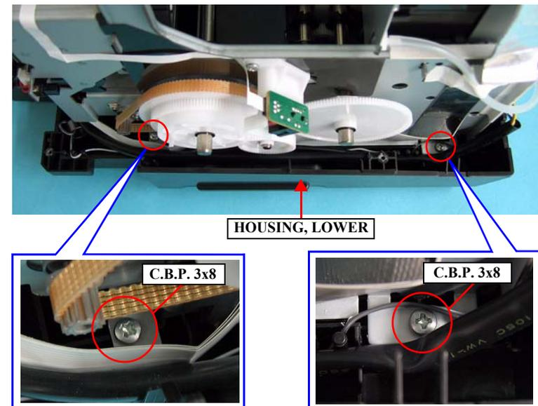
Figure 4-128. Removing the screws from the HOUSING, LOWER
