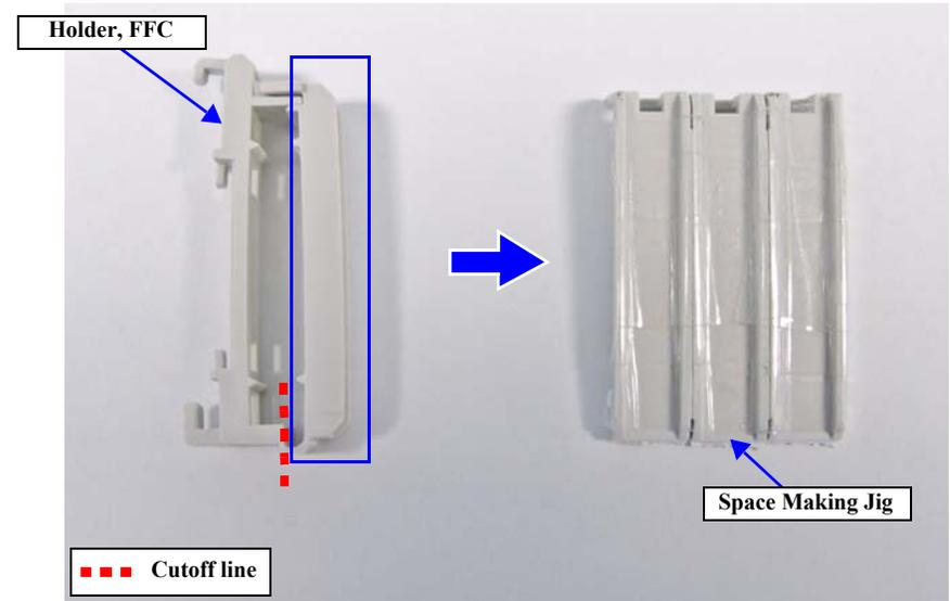
Figure 4-104. Preparing the Space Making Jig
