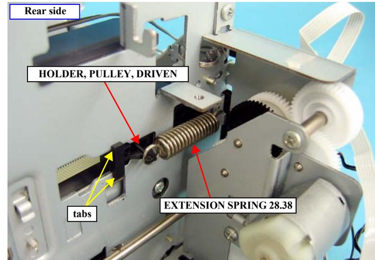
Figure 4-152. Removing the EXTENSION SPRING 28.38 and HOLDER, PULLEY, DRIVEN
