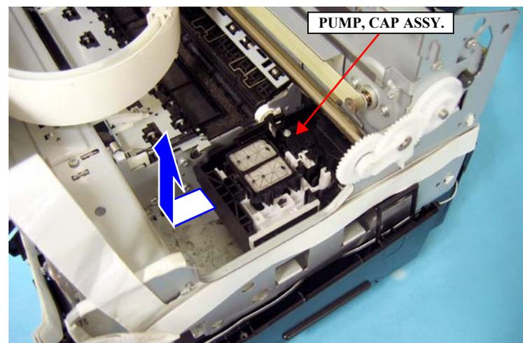
Figure 4-78. Removing the PUMP, CAP ASSY.
