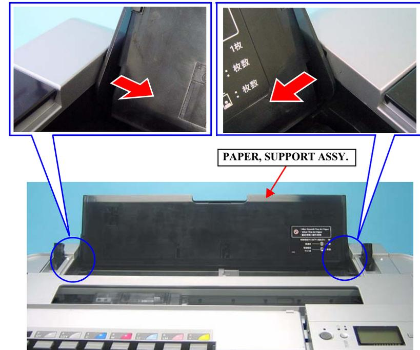
Figure 4-13. Removing the PAPER SUPPORT ASSY.
