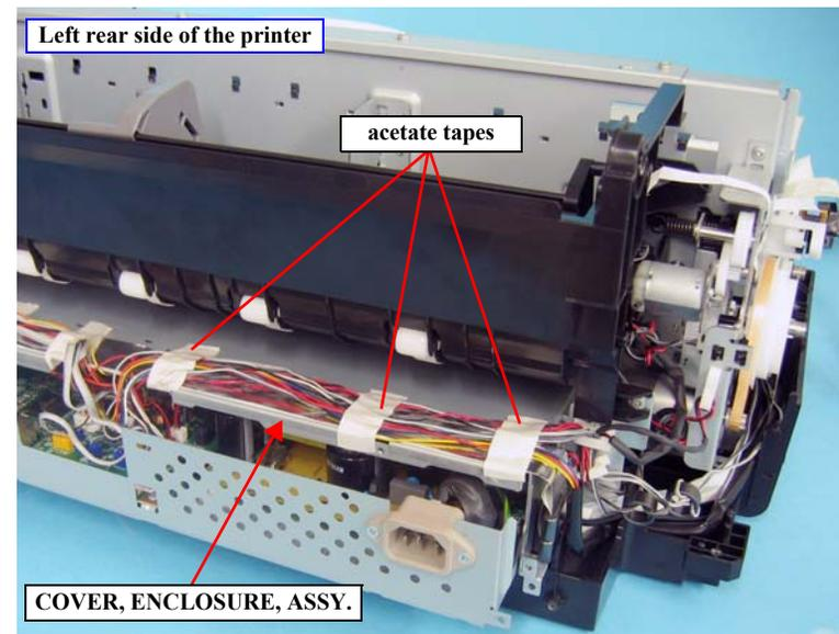
Figure 4-48. Releasing the LOCK, COVER, ASSY. Cables (2)
