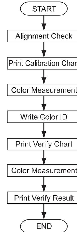
**Figure 5-38. Adjustment Workflow**
