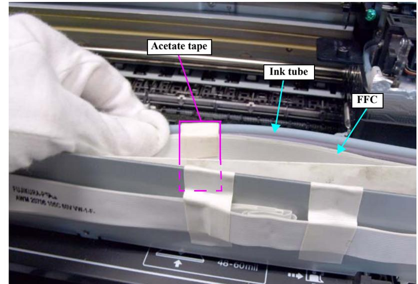
Figure 4-102. Releasing the Ink Tube and FFCs
