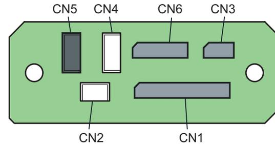
Figure 4-36. Connector Layout of the BOARD ASSY., SUB
