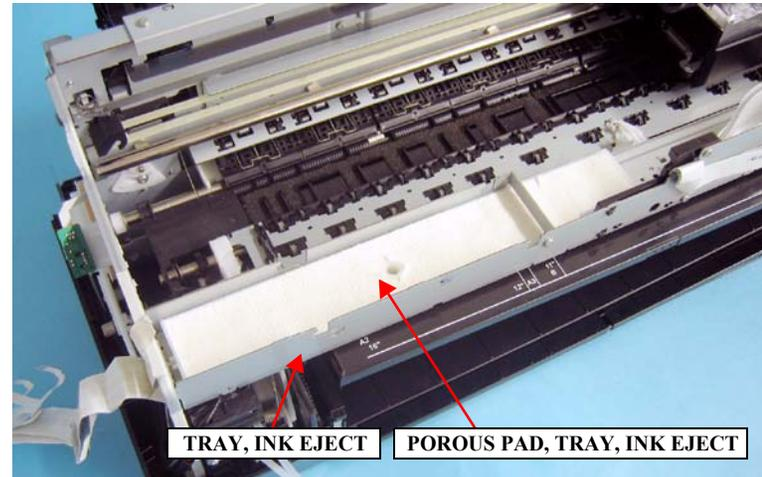
Figure 4-88. Removing the POROUS PAD, TRAY, INK EJECT
