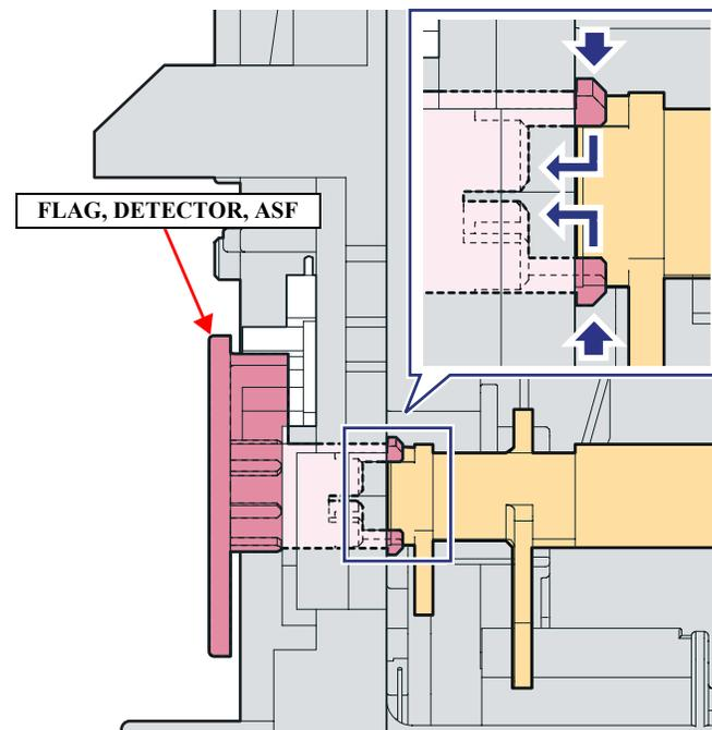
Figure 4-154. Removing the FLAG, DETECTOR, ASF
