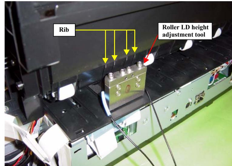
Figure 5-6. Setting the Roller LD Height Adjustment Tool
