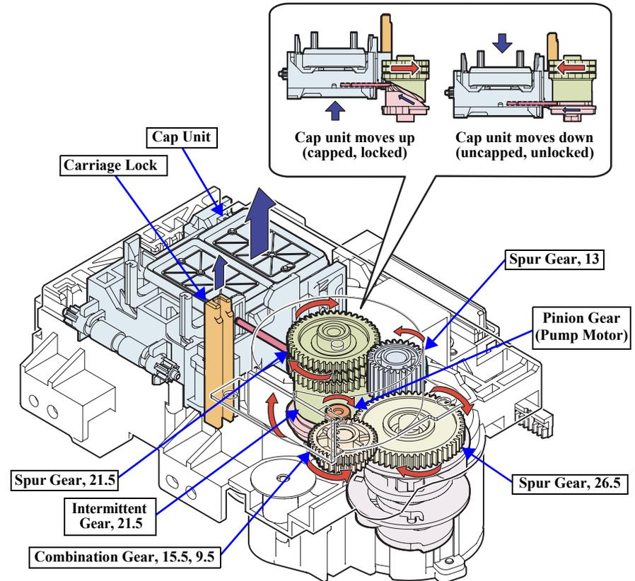
Figure 2-12. Cap Unit/Carriage Lock Mechanism
