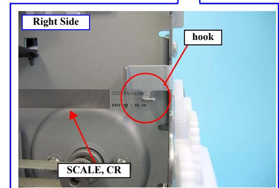
Figure 4-54. Removing the SCALE, CR (1)
