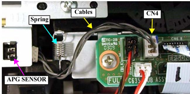
4. Remove the two screws that secure the BOARD ASSY., SUB to the CARRIAGE, ASSY., and remove the BOARD ASSY., SUB.
