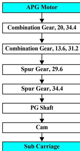
Figure 2-16. Drive Transmission Path
