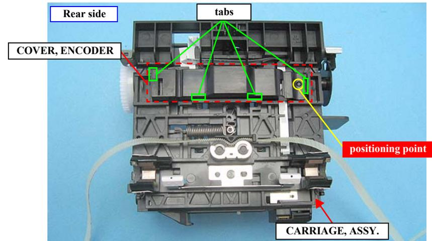
Figure 4-140. Removing the COVER, ENCODER
