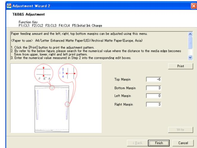
Figure 5-68. [T&B&S Adjustment] Screen
