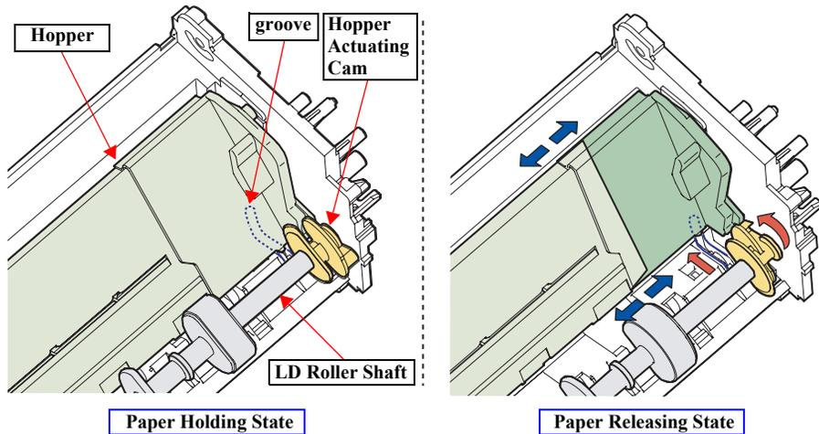
Figure 2-23. Releasing the Back End of Paper
