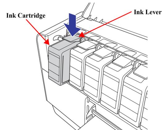
Figure 4-4. Removing the Ink Cartridges
