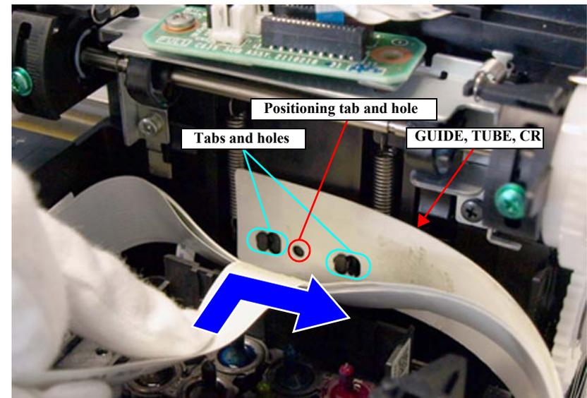
Figure 4-106. Installing the GUIDE, TUBE, CR
