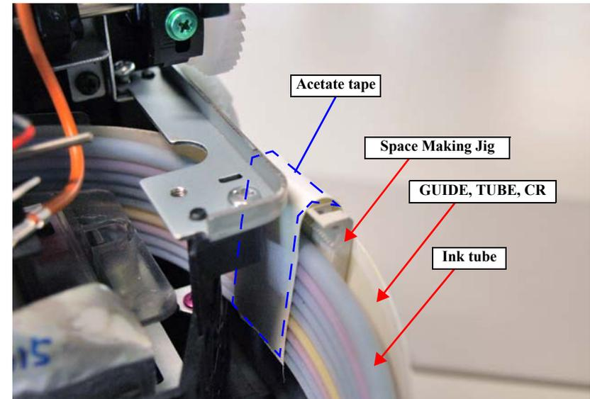
Figure 4-115. Temporarily Securing with Acetate Tape
