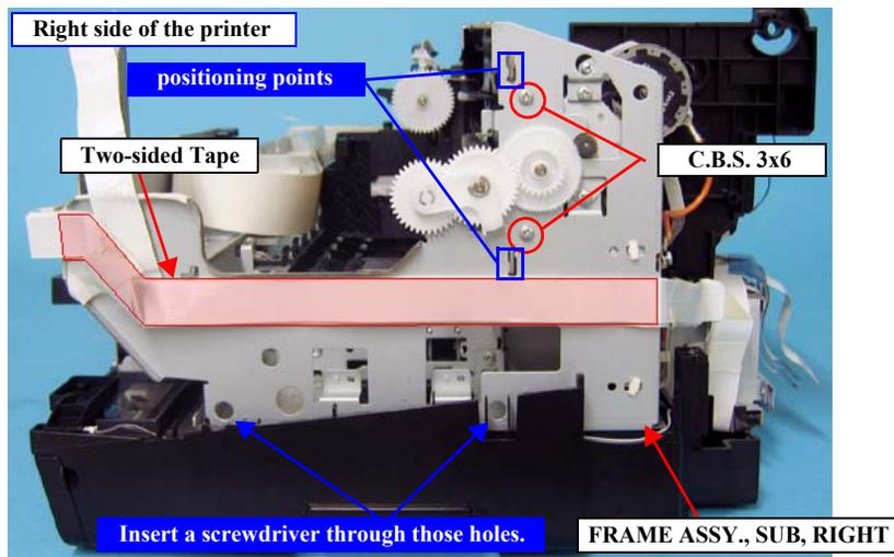
Figure 4-137. Removing the FRAME ASSY., SUB, RIGHT
