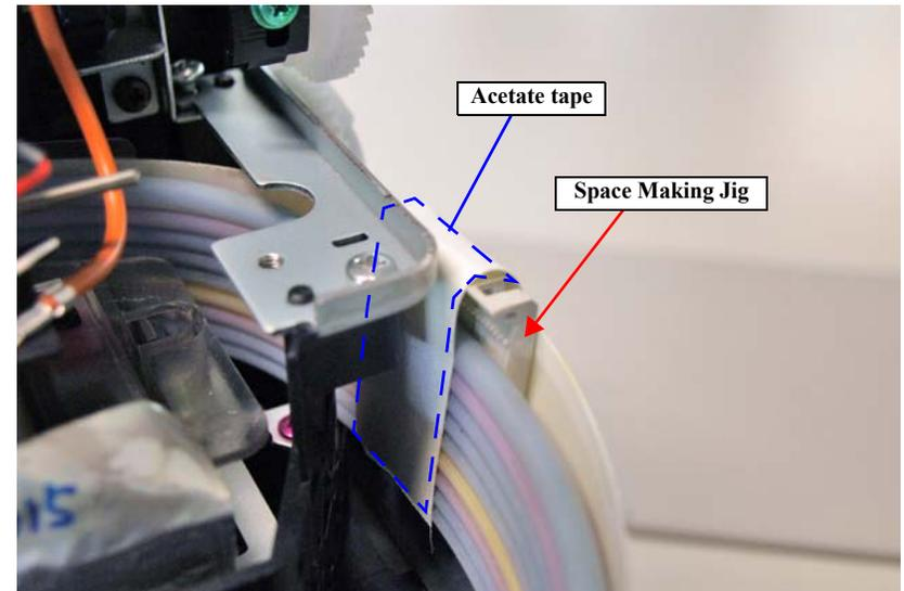
Figure 4-119. Removing the Space Making Jig
