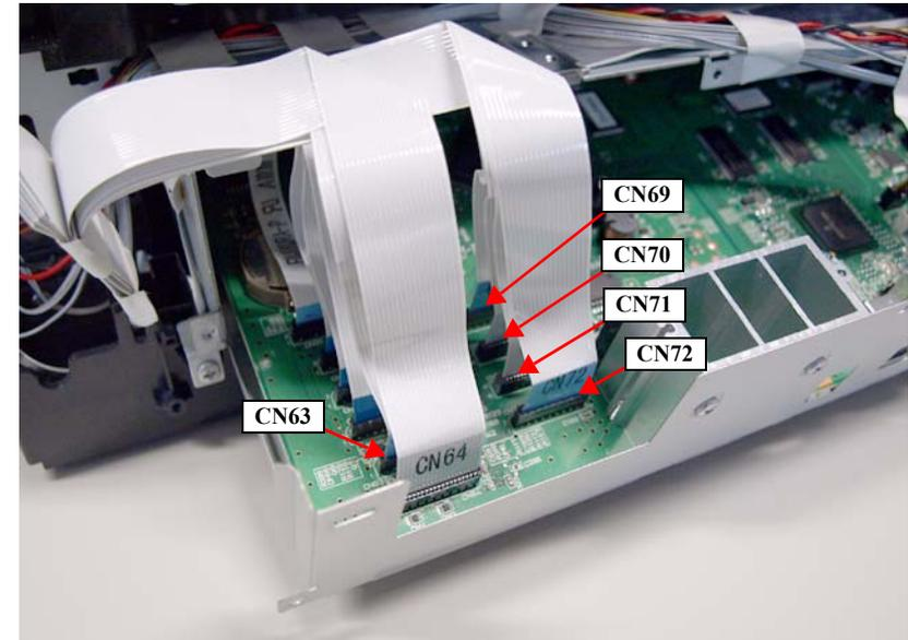
Figure 4-100. Disconnecting the Cables
