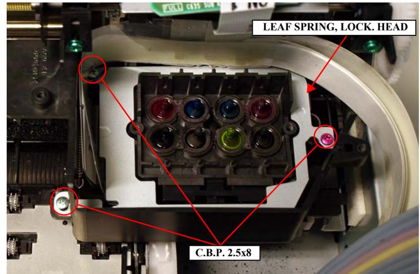
Figure 4-107. Securing the LEAF SPRING, LOCK, HEAD
