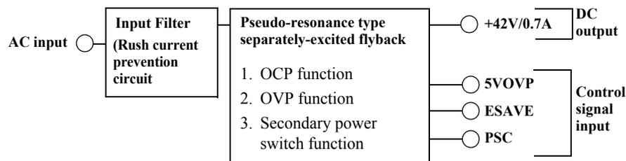
Figure 2-34. C635 Power Supply Board Block Diagram
