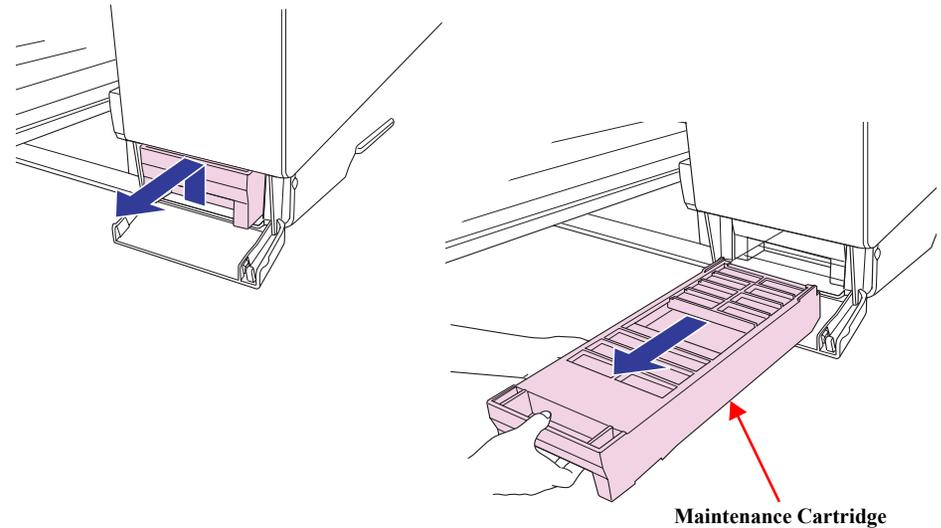
Figure 4-6. Removing the Maintenance Cartridge
