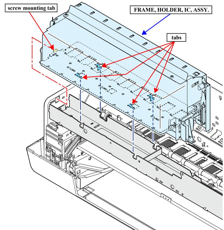
Figure 4-84. Removing the FRAME, HOLDER, IC, ASSY.
