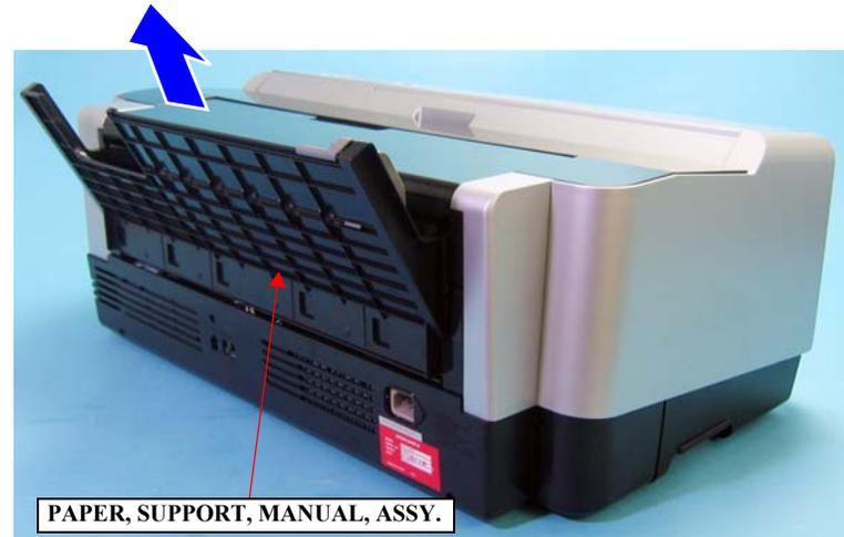
Figure 4-12. Removing the PAPER, SUPPORT, MANUAL, ASSY.
