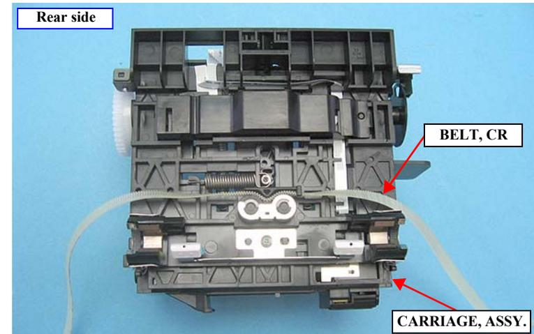
Figure 4-146. Removing the BELT, CR
