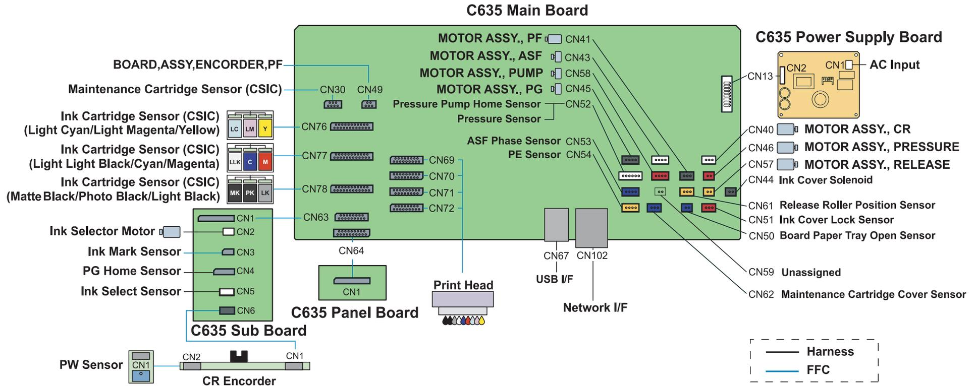
Figure 7-1. Block Diagram
