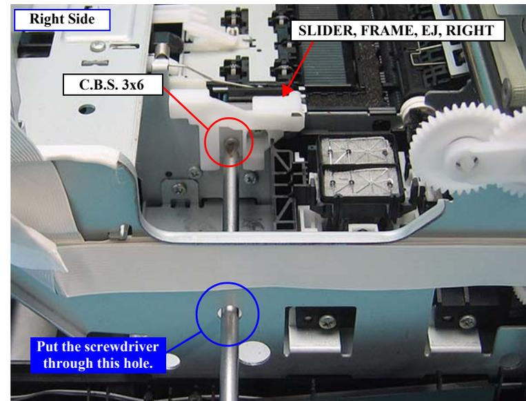
Figure 4-68. Removing the SLIDER, FRAME, EJ, RIGHT
