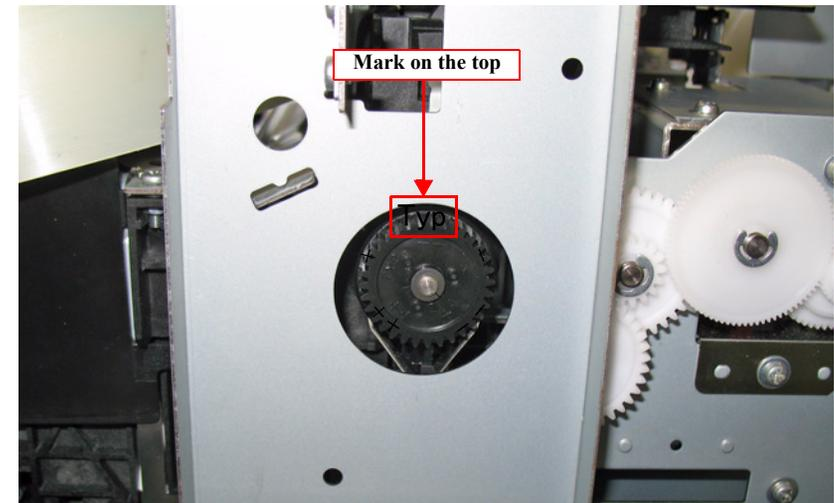
Figure 4-31. APG cam position checking point
