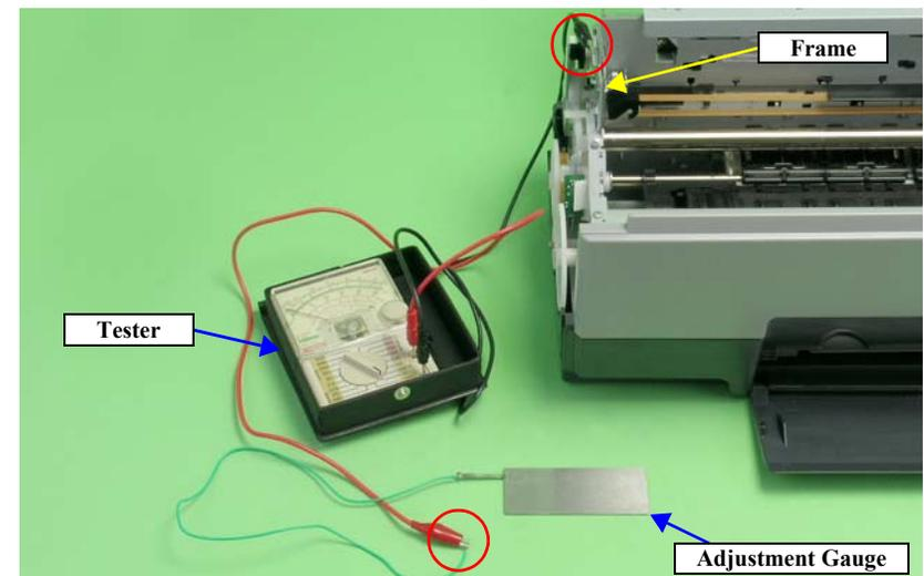
Figure 4-11. Connecting the Tester
