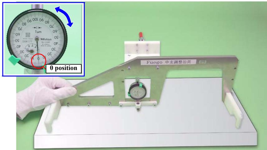
Figure 4-20. Setting the PF Roller Shaft Position Adjustment Jig (1)
