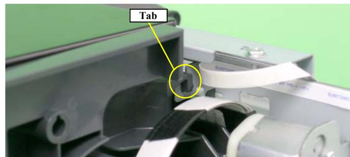
Figure 3-88. Reinstalling the ASF Assy
