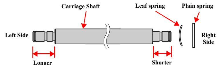
Figure 3-76. Reinstalling the Carriage Shaft
