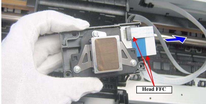
Figure 3-51. Removing the Printhead (2)
