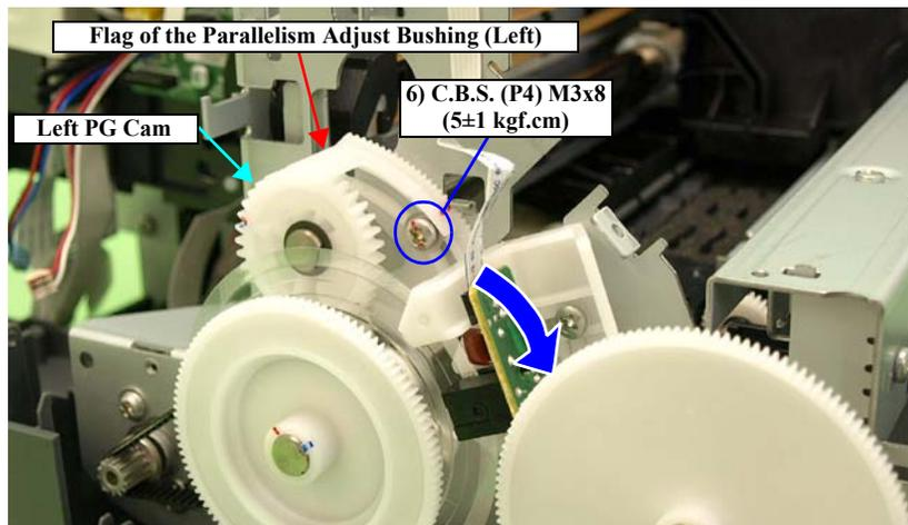
Figure 3-67. Rotating the Left Parallelism Adjust Bushing
