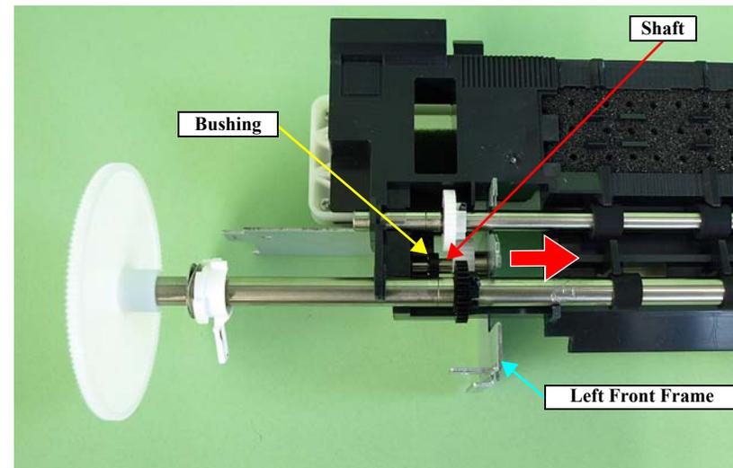
Figure 3-122. Removing the Front Paper Guide/Paper EJ Rollers (2)
