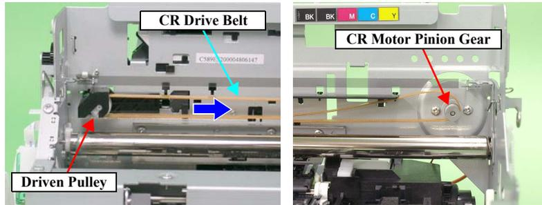
Figure 3-142. Removing the CR Motor
