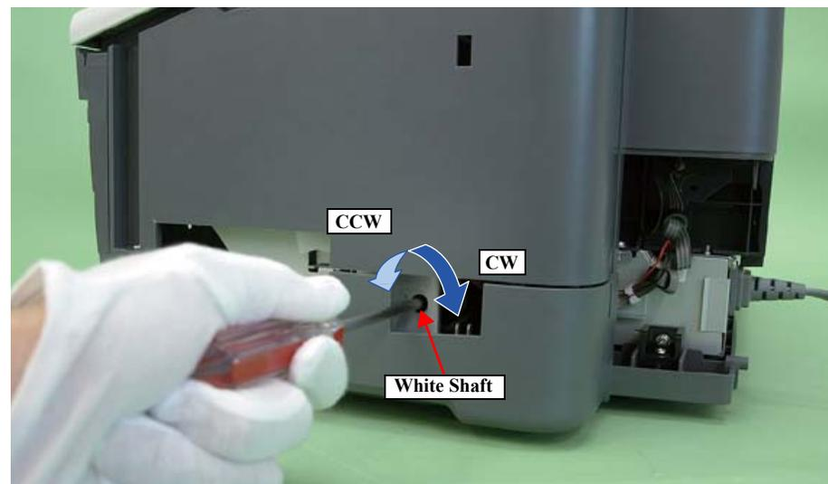
Figure 3-8. Release the Carriage Lock
