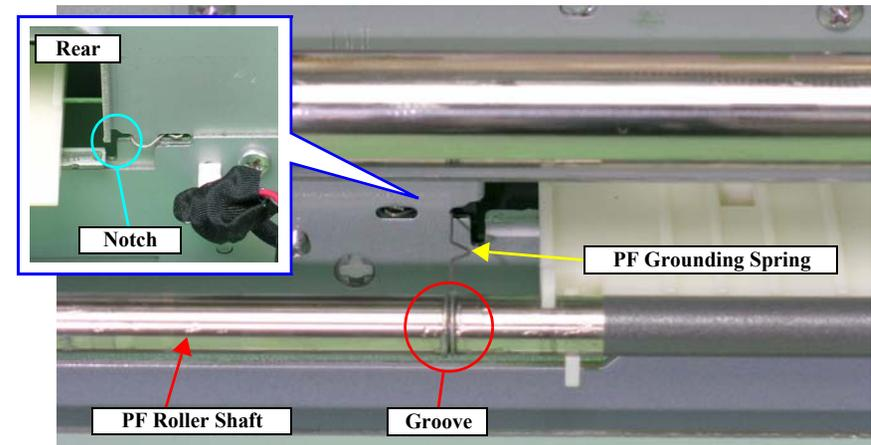
Figure 3-127. Removing the PF Grounding Spring
