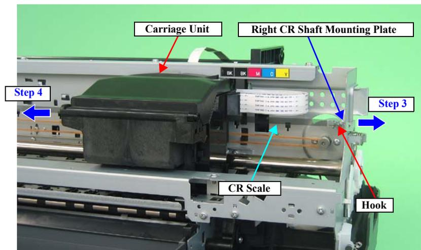
Figure 3-39. Pulling out the CR Scale
