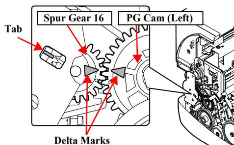
Figure 3-38. Phase Aligning
