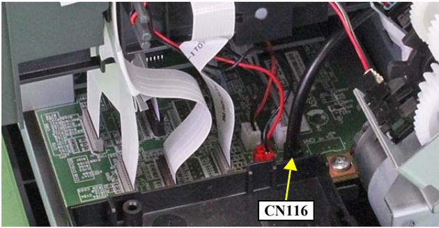
2. Check the PF Motor connector cable for damages.<br>3. Check if the PF Motor operates normally. | 1. Connect the PF Motor connector cable to the Main Board connector CN116.<br><br>2. Replace the PF Motor with a new one.<br>3. Replace the PF Motor with a new one. |
