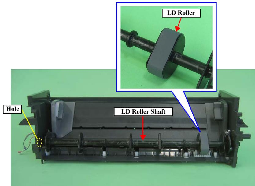
Figure 3-92. Removing the LD Roller (4)
