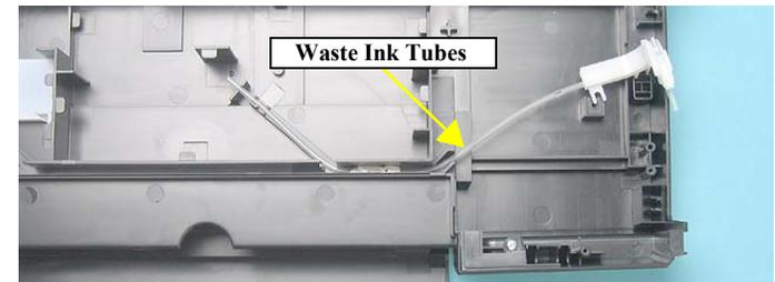
Figure 3-103. Positions of Waste Ink Tubes
