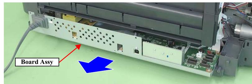
Figure 3-32. Removing the Board Assy (2)
