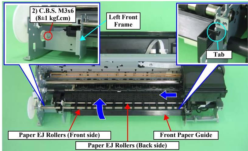
Figure 3-121. Removing the Front Paper Guide/Paper EJ Rollers (1)
