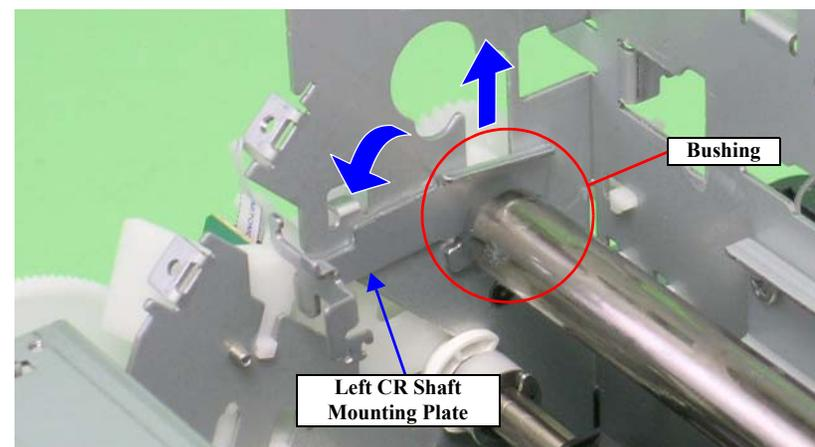
Figure 3-70. Removing the Left CR Shaft Mounting Plate
