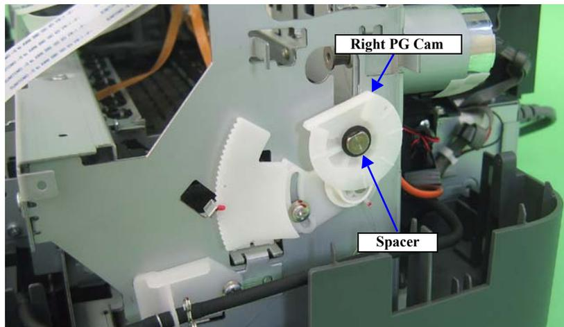
Figure 3-72. Removing Right PG Cam
