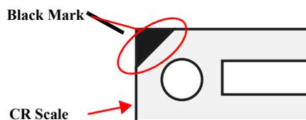
Figure 3-44. Reinstalling the CR Scale (2)
