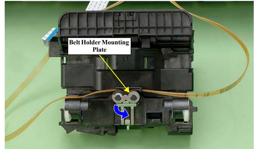
Figure 3-78. Removing the Belt Holder Mounting Plate
