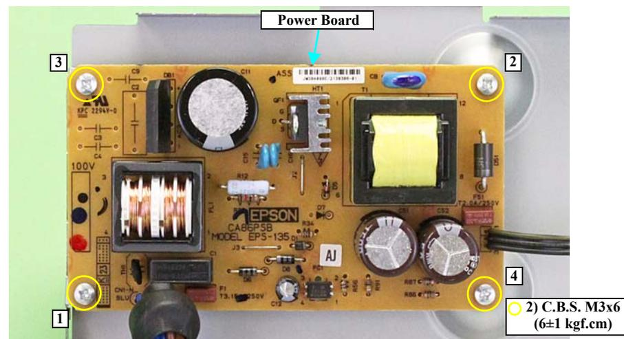
Figure 3-34. Removing the Power Board
