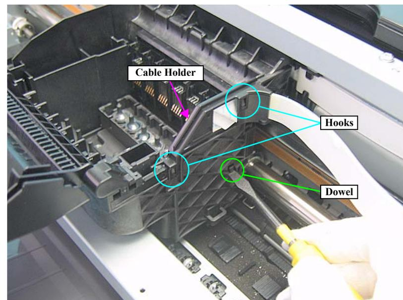
Figure 3-46. Removing the Adapter Guide Holder (1)
