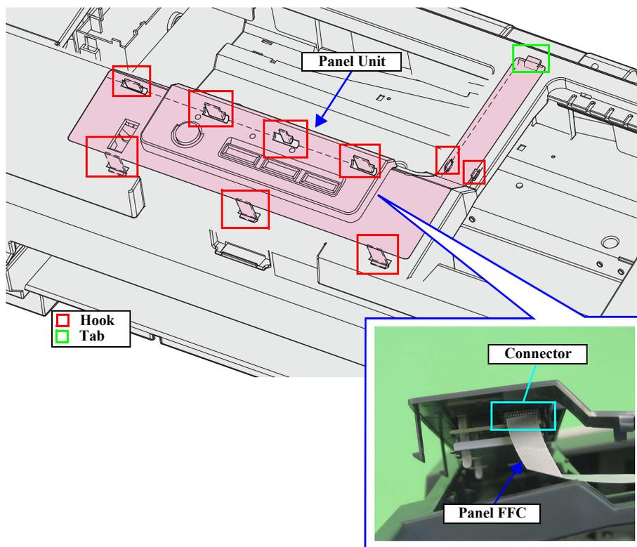
Figure 3-20. Removing the Panel Unit (2)
