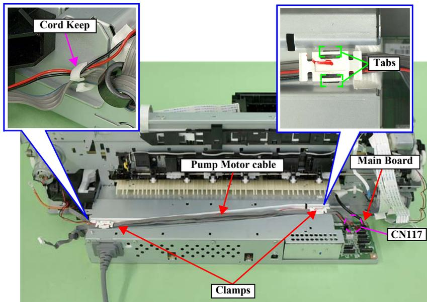
Figure 3-109. Removing the Pump Motor cable
