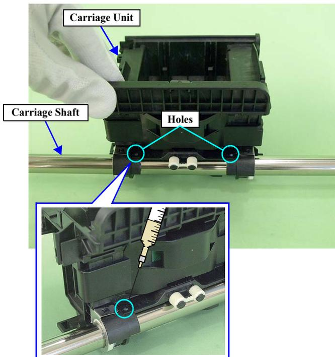
Figure 5-19. Lubricating the Carriage Shaft (1)
