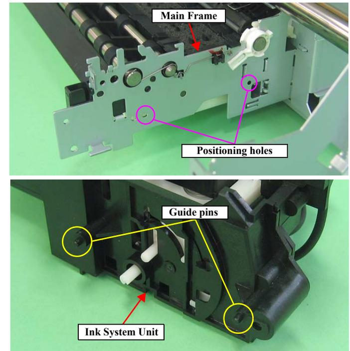
Figure 3-116. Reinstalling the Ink System Unit
