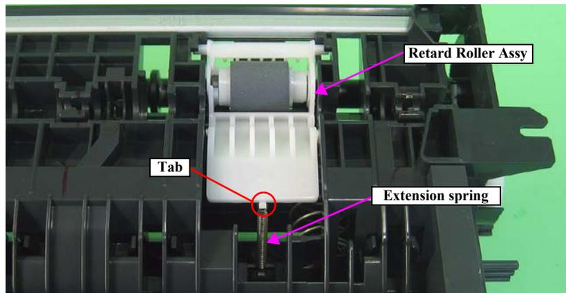
Figure 3-96. Removing the Retard Roller Assy (2)
