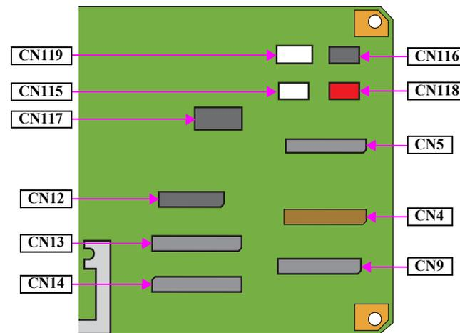
Figure 3-31. Connector Layout of the Main Board (130 Digit Side)
