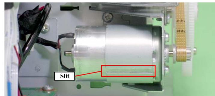
Figure 3-146. Reinstalling the PF Motor
