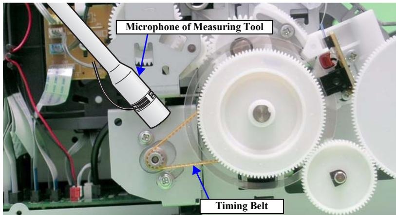
Figure 4-9. Microphone Position
