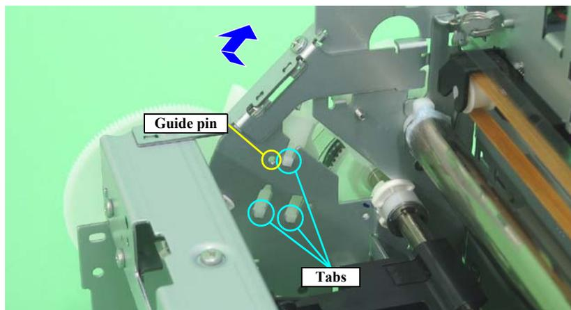
Figure 3-151. Removing the PF Encoder Sensor Holder
