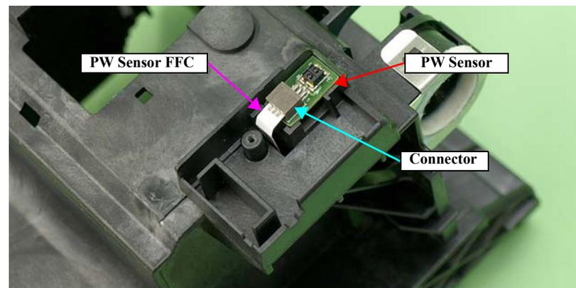
Figure 3-154. Removing the PW Sensor
