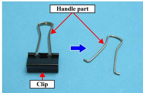
Figure 3-9. Method for making Adapter Guide Holder Removal Tool (1)
