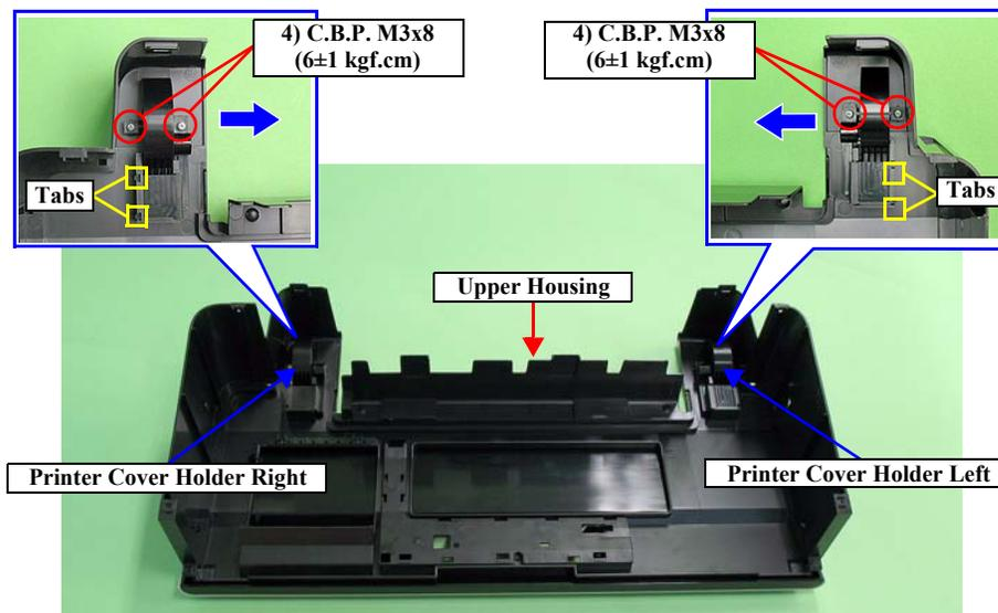
Figure 3-27. Removing the Printer Cover Holder Left/Right
