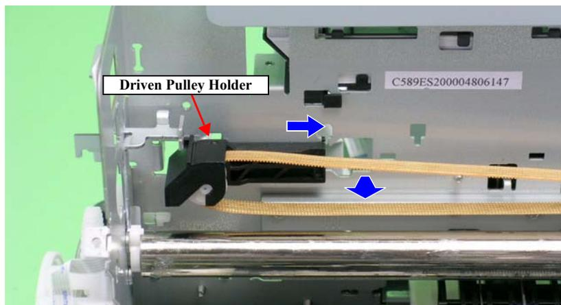
Figure 3-64. Removing the Driven Pulley Holder
