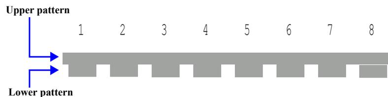
Figure 4-6. PF (bottom margin area) Adjustment Printout Pattern
