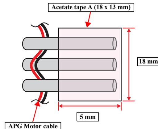
Figure 3-36. Applying the Acetate tape A
