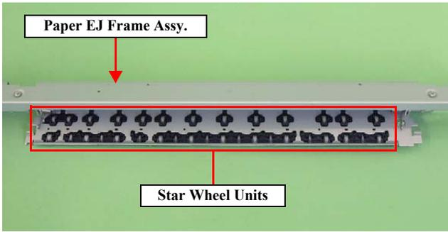
2. Check the Paper EJ Frame Assy for deformation or damages. | 1. Securely install the Star Wheel Units to the Paper EJ Frame Assy.                           |
