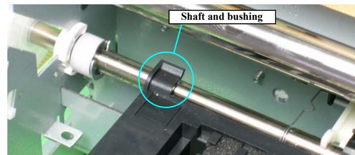
Figure 3-123. The PF Roller Shaft and the bushing of the Front Paper Guide
