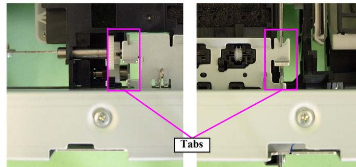
Figure 3-108. Reinstalling the Paper EJ Frame Assy
