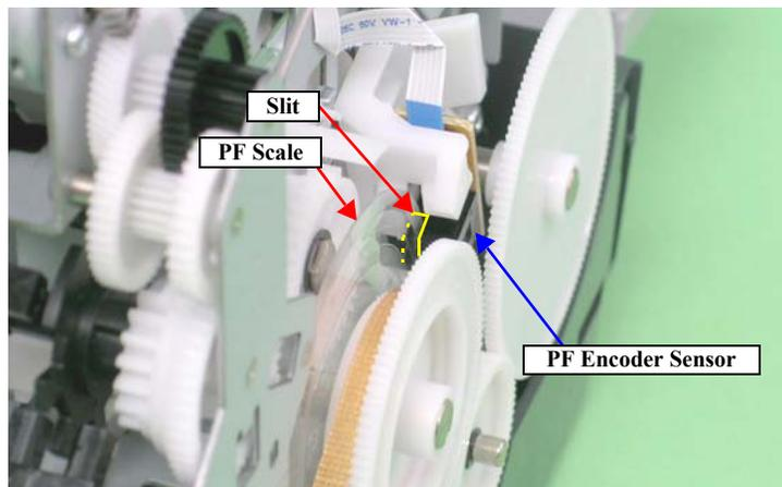
Figure 3-152. Reinstalling the PF Encoder Sensor Holder
