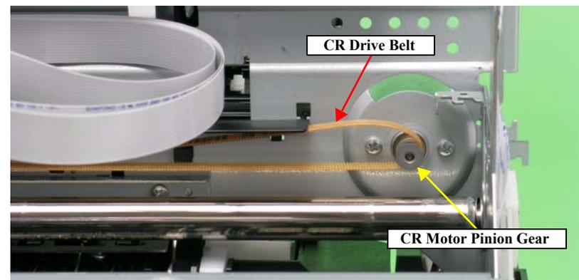
Figure 3-65. Removing the CR Drive Belt
