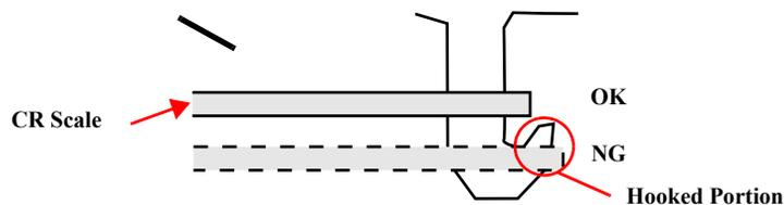
Figure 3-45. Reinstalling the CR Scale (3)
