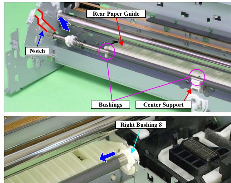
Figure 3-132. Removing the PF Roller Shaft
