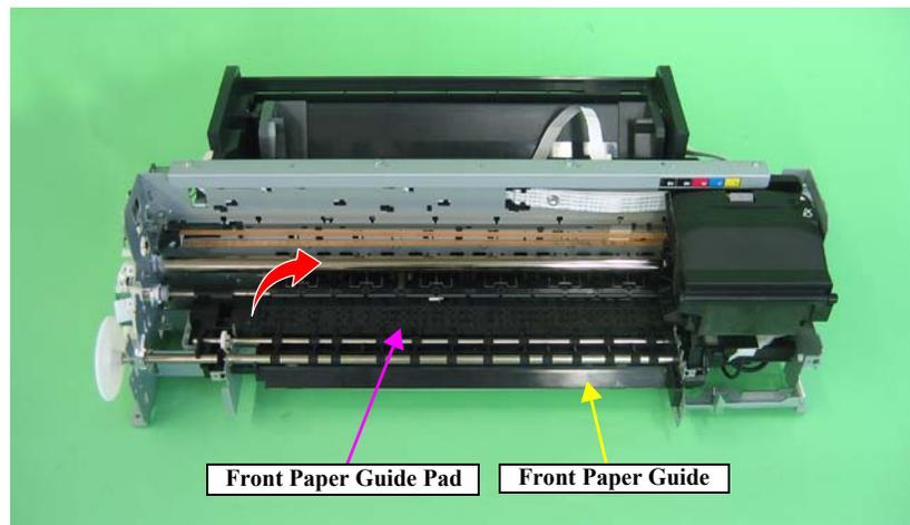
Figure 3-99. Removing the Front Paper Guide Pad
