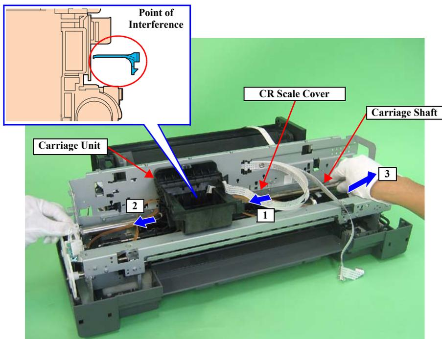
Figure 3-75. Removing the Carriage Shaft
