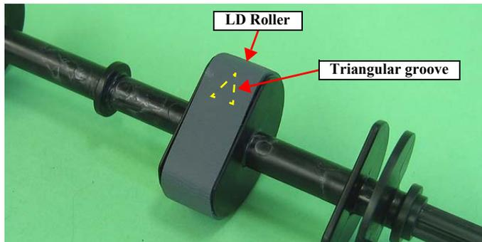
Figure 3-93. Reinstalling the LD Roller
