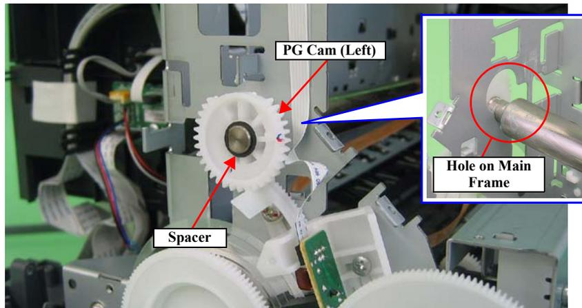
Figure 3-71. Removing Left PG Cam
