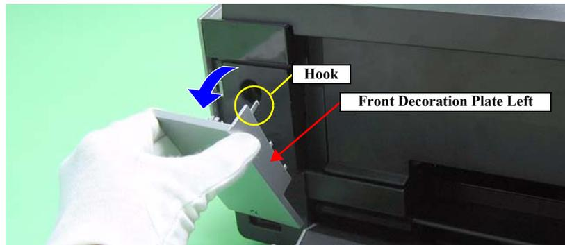
Figure 3-15. Removing the Front Decoration Plate Left/Right
