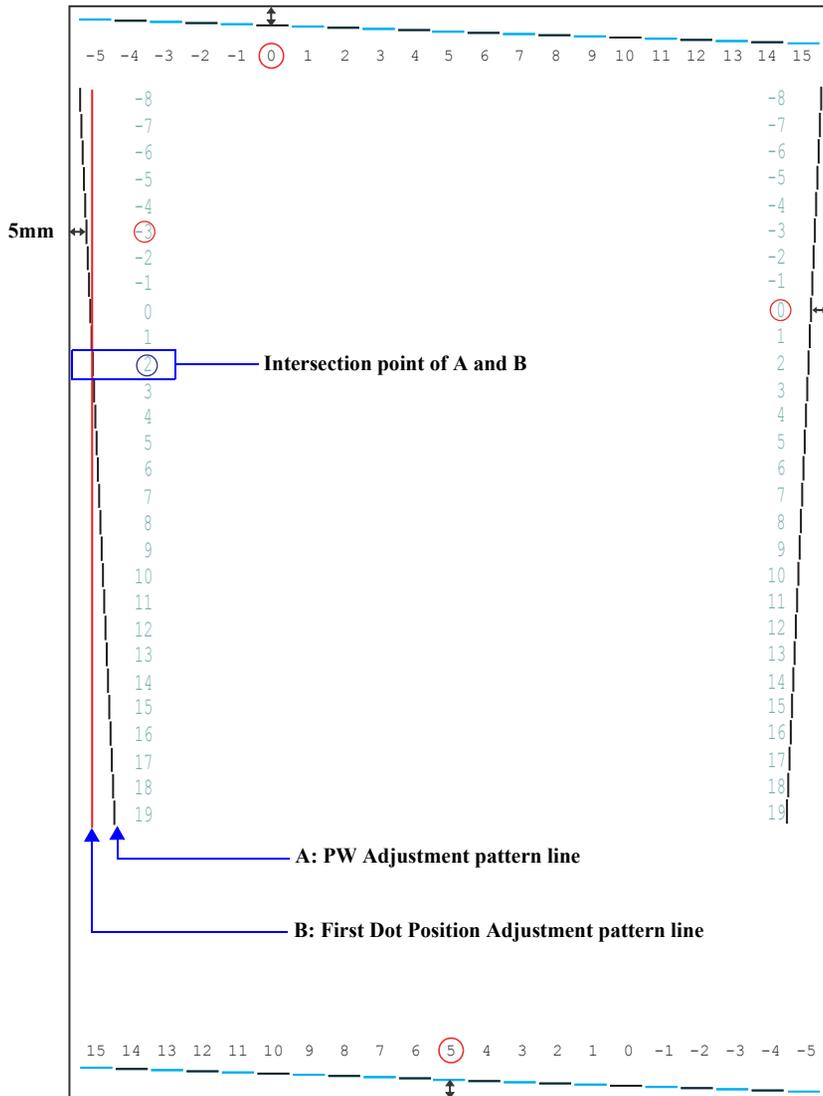
Figure 4-2. PW Adjustment Pattern/First Dot Position Adjustment Pattern
