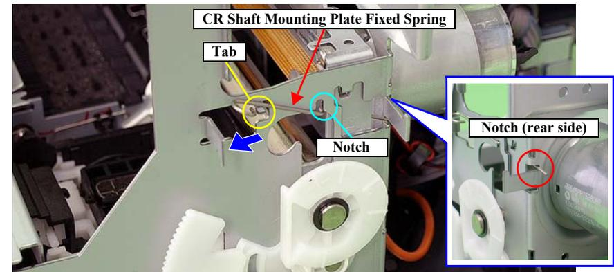
Figure 3-62. Removing CR Shaft Mounting Plate Fixed Spring
