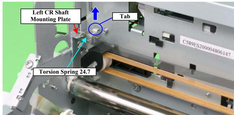
Figure 3-40. Removing the Torsion Spring 24.7 (1)
