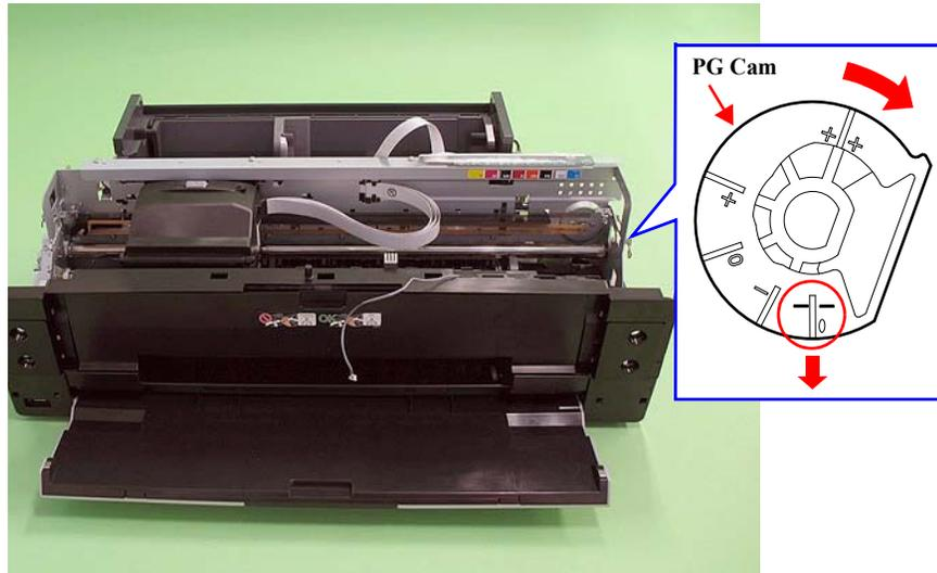
Figure 4-15. Markings of the PG Cam
