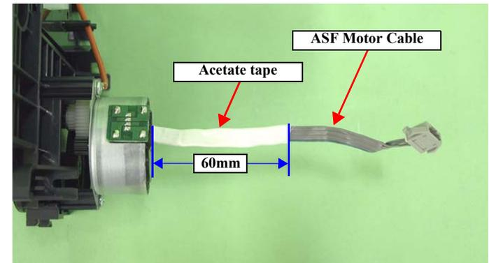
Figure 3-148. Attaching acetate tape
