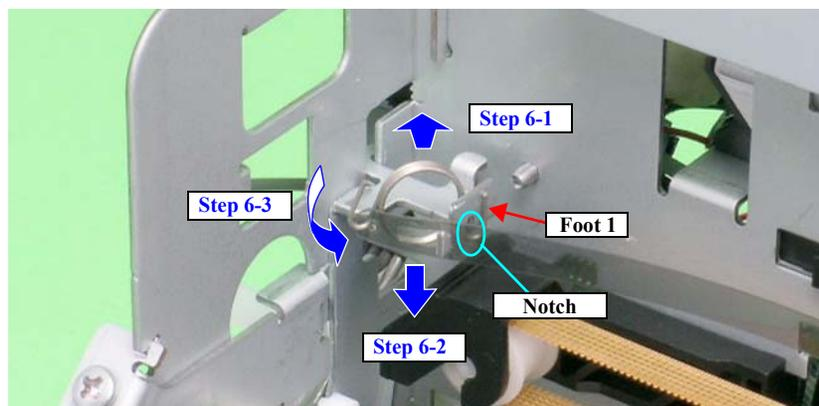
Figure 3-41. Removing the Torsion Spring 24.7 (2)
