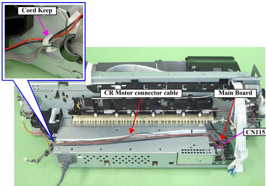
Figure 3-139. Removing the CR Motor connector cable
