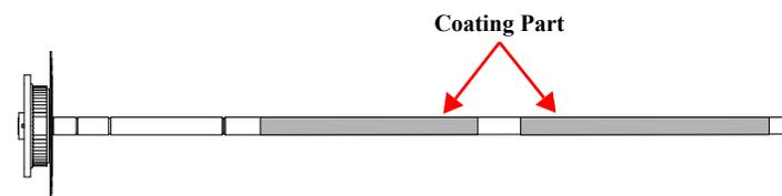
Figure 3-131. Handling the PF Roller Shaft
