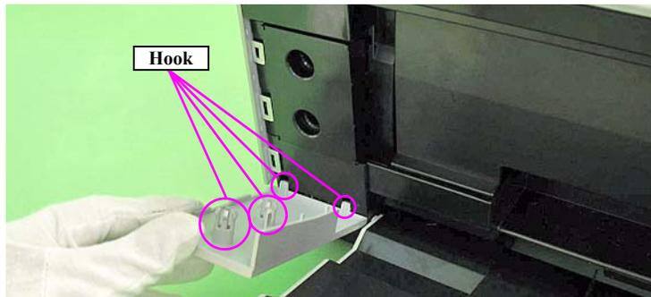
Figure 3-16. Reinstalling the Front Decoration Plate Left/Right
