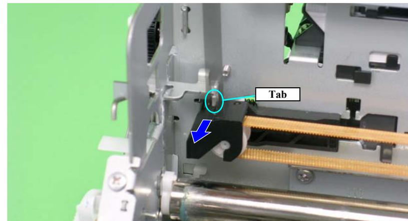
Figure 3-42. Removing the CR Scale
