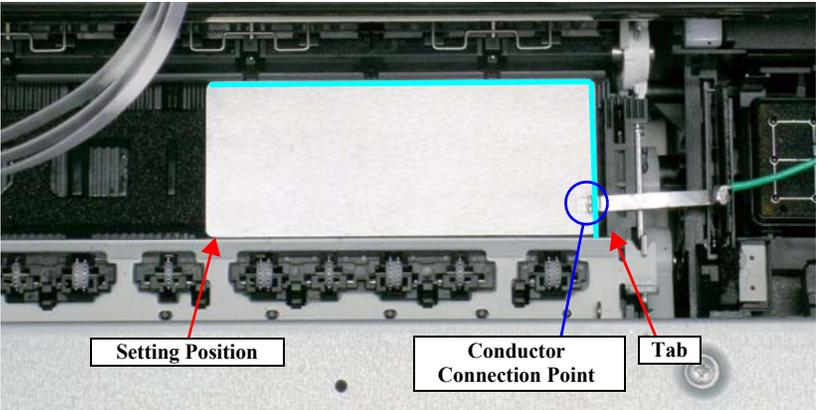
Figure 4-17. Setting the Adjustment Gauge
