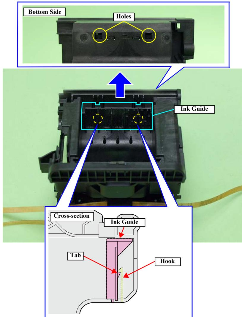
Figure 3-77. Removing the Ink Guide
