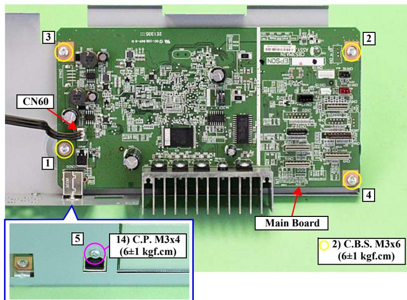
Figure 3-33. Removing the Main Board
