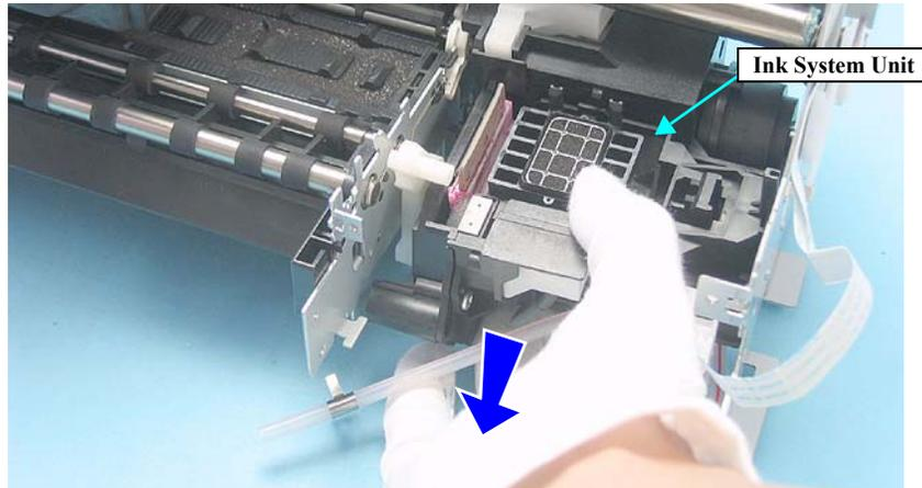
Figure 3-115. Removing the Ink System Unit
