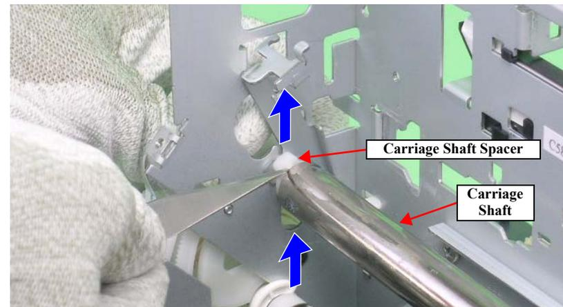
Figure 3-69. Removing the Carriage Shaft Spacer
