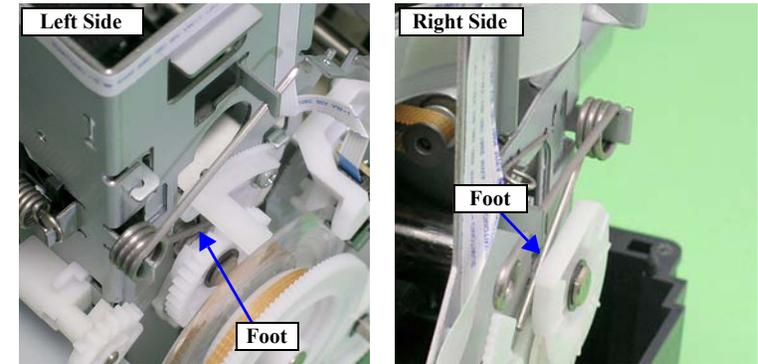
Figure 3-61. Reinstalling PG Torsion Springs
