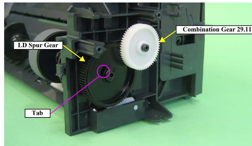
Figure 3-89. Removing the LD Roller (1)
