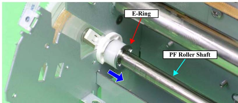
Figure 3-130. Removing the Left Bushing 8
