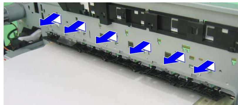
Figure 3-138. Removing the Upper Paper Guide Assy
