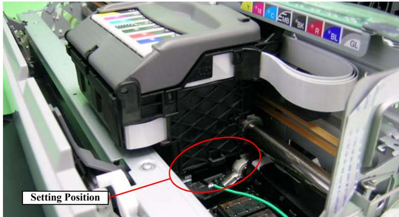
Figure 4-18. Moving the Carriage Unit
