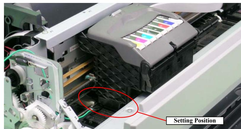
Figure 4-14. Moving the Carriage Unit
