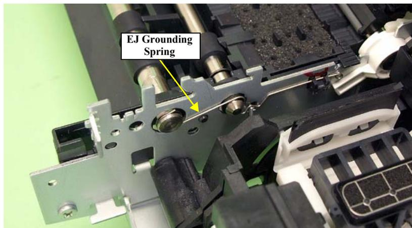
Figure 3-117. Removing the EJ Grounding Spring
