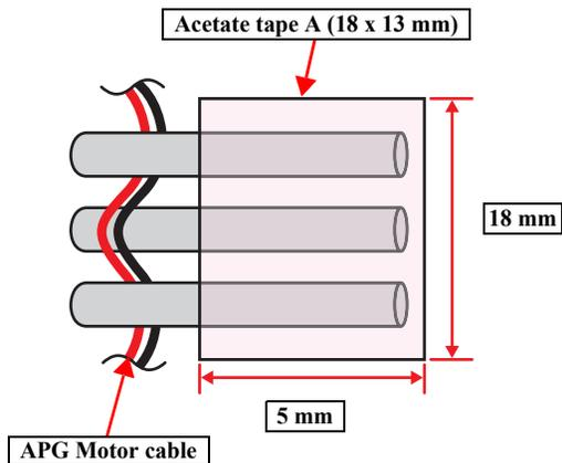
Figure 3-84. Applying the Acetate tape A
