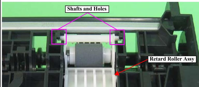
Figure 3-97. Reinstalling the Retard Roller Assy
