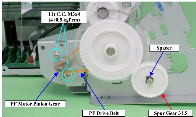
Figure 3-126. Removing the PF Drive Belt and Spur Gear 31.5
