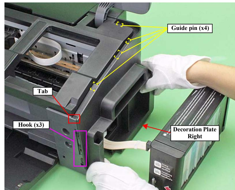
Figure 3-23. Removing the Decoration Plate Left/Right (2)
