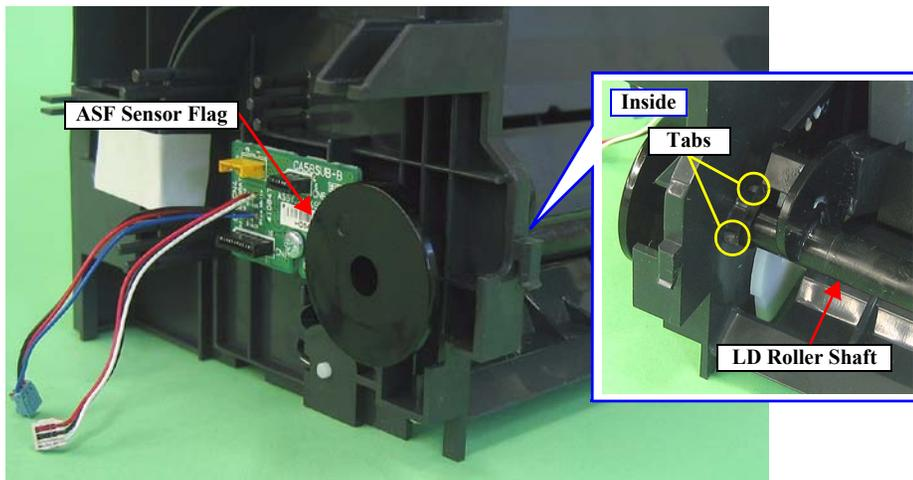
Figure 3-90. Removing the LD Roller (2)
