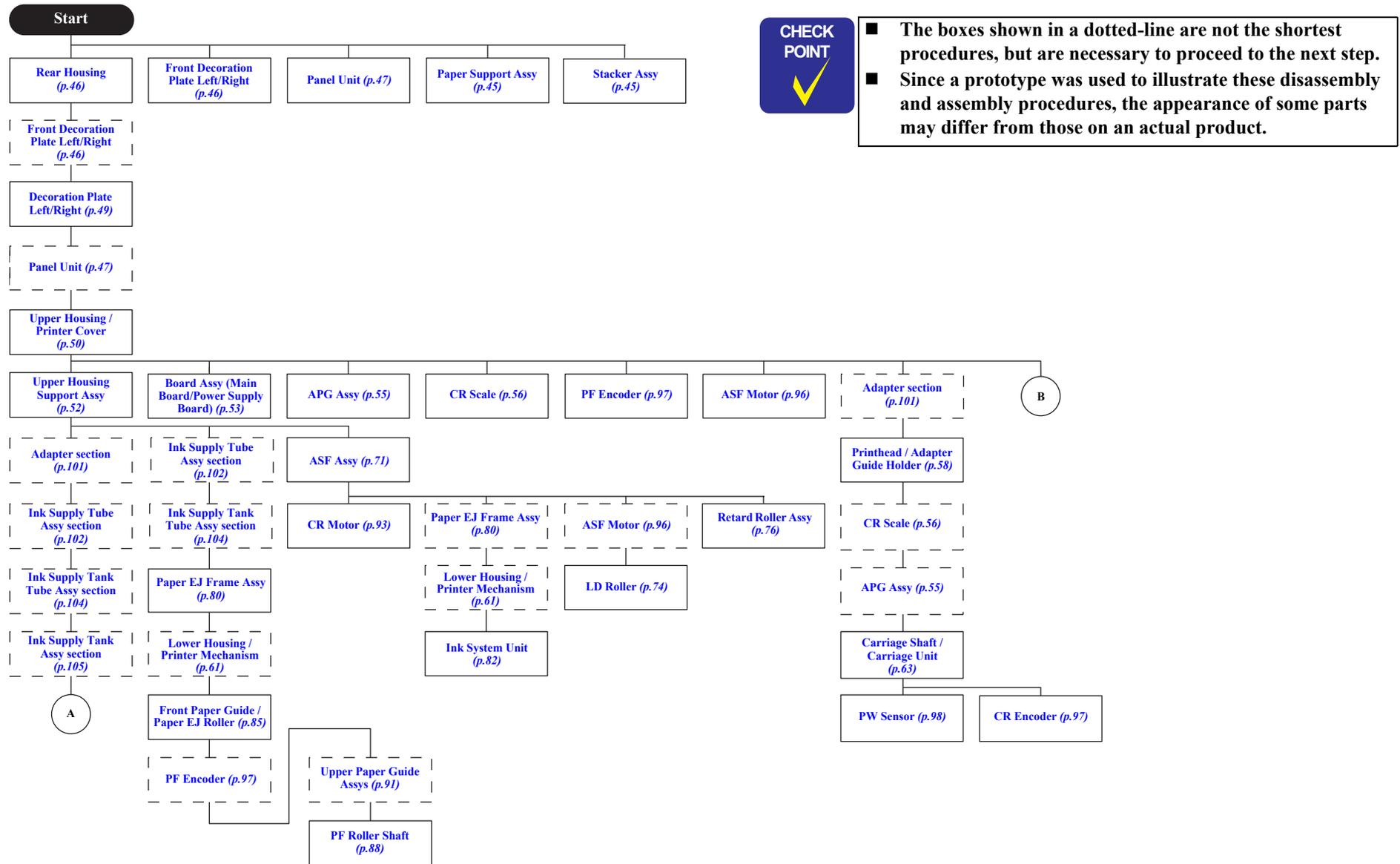
Figure 3-11. Disassembly Flowchart (1)
