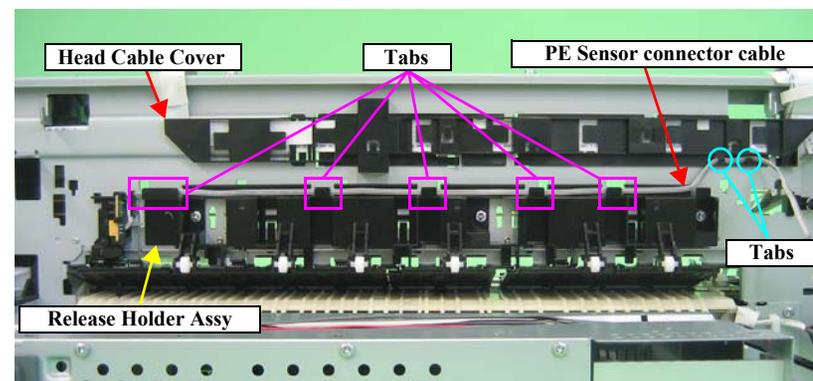
Figure 3-155. Releasing the Cables
