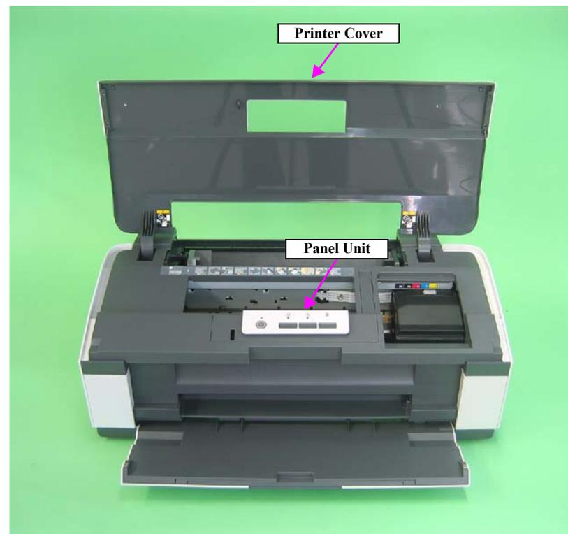
Figure 3-19. Removing the Panel Unit (1)
