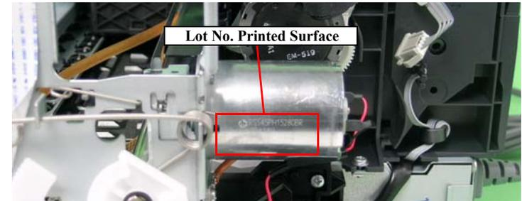
Figure 3-144. Reinstalling the CR Motor
