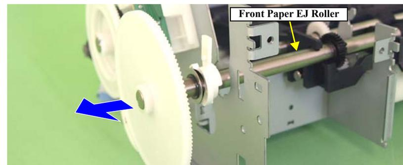
Figure 3-120. Removing the Left Bushing 8
