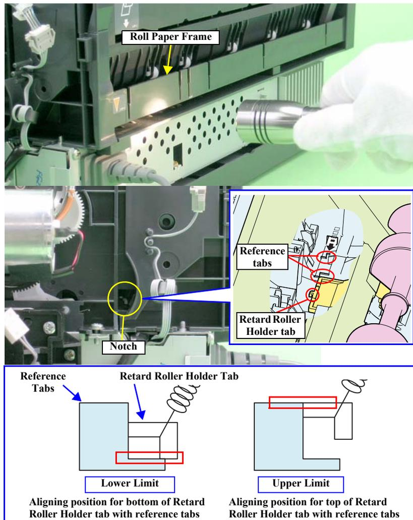
Figure 4-28. Aligning the Position of the Guide Roller LD (0 Digit Side)
