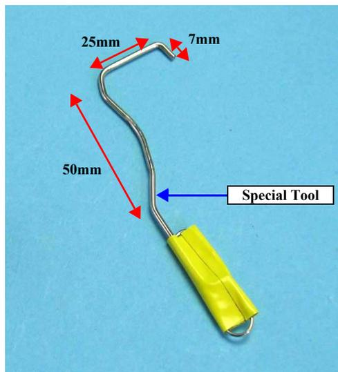
Figure 3-10. Method for making Adapter Guide Holder Removal Tool (2)
