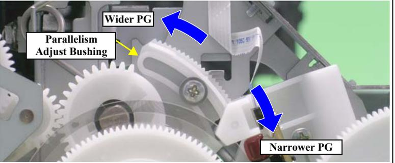
Figure 4-16. Relationship between Parallelism Adjust Bushing and PG
