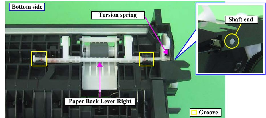
Figure 3-95. Removing the Retard Roller Assy (1)
