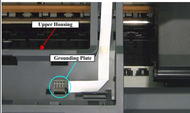
Figure 3-26. Routing the Panel FFC
