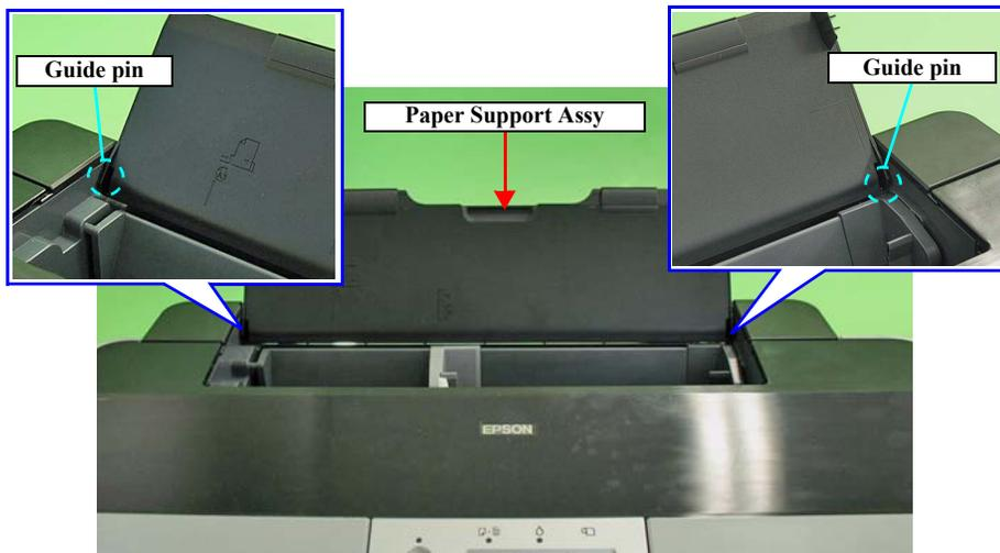
Figure 3-13. Removing the Paper Support Assy
