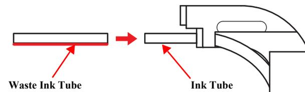
Figure 3-55. Installing the Ink Tubes
