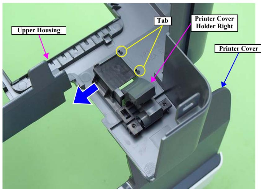
Figure 3-28. Removing the Printer Cover
