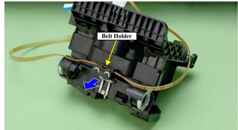
Figure 3-79. Removing the Belt Holder
