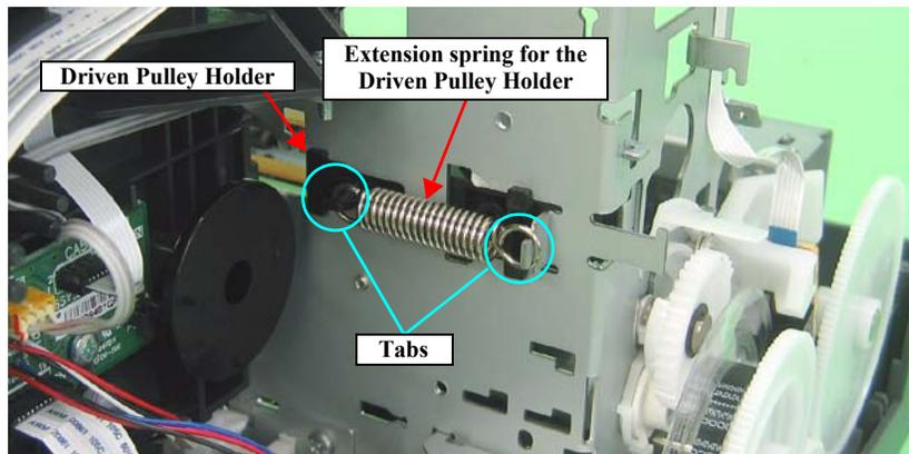
Figure 3-63. Removing the Extension Spring for the Driven Pulley Holder
