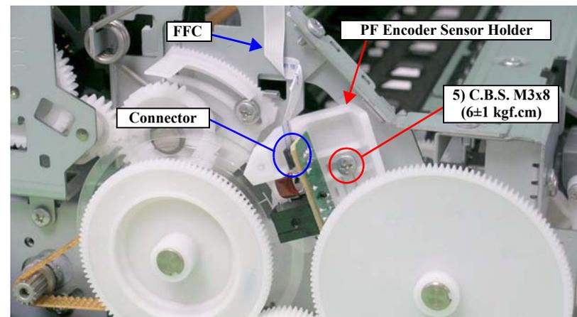
Figure 3-150. Removing the FFC and the Screw that Secures the PF Encoder Sensor Holder
