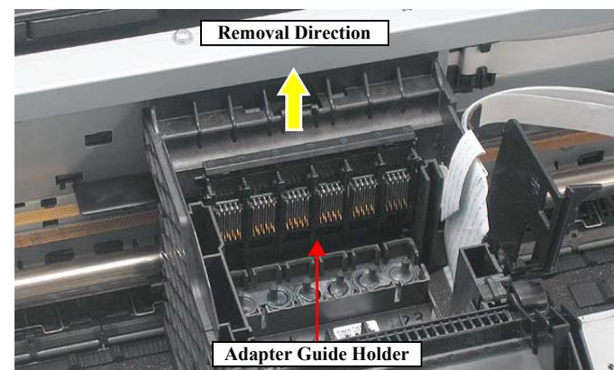
Figure 3-49. Removing the Adapter Guide Holder (4)
