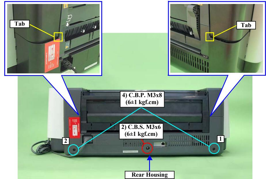
Figure 3-17. Removing the Rear Housing
