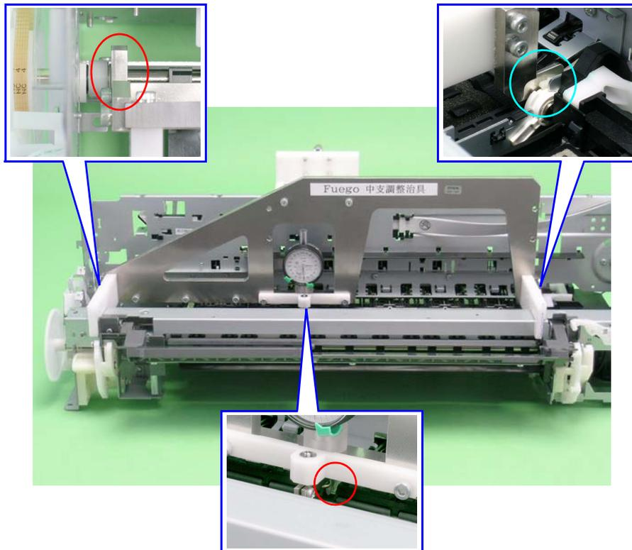
Figure 4-22. Setting the PF Roller Shaft Position Adjustment Jig (2)
