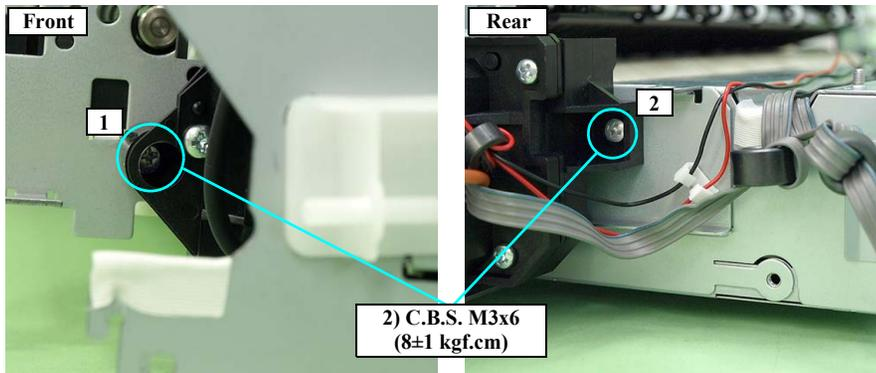
Figure 3-112. Screws that Secure the Ink System Unit
