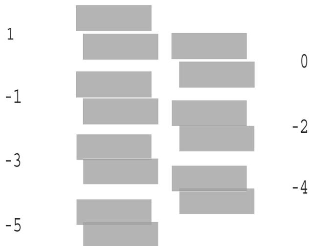
Figure 4-5. PF (standard print area) Adjustment Printout Pattern
