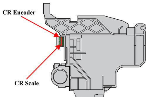
Figure 3-43. Reinstalling the CR Scale (1)
