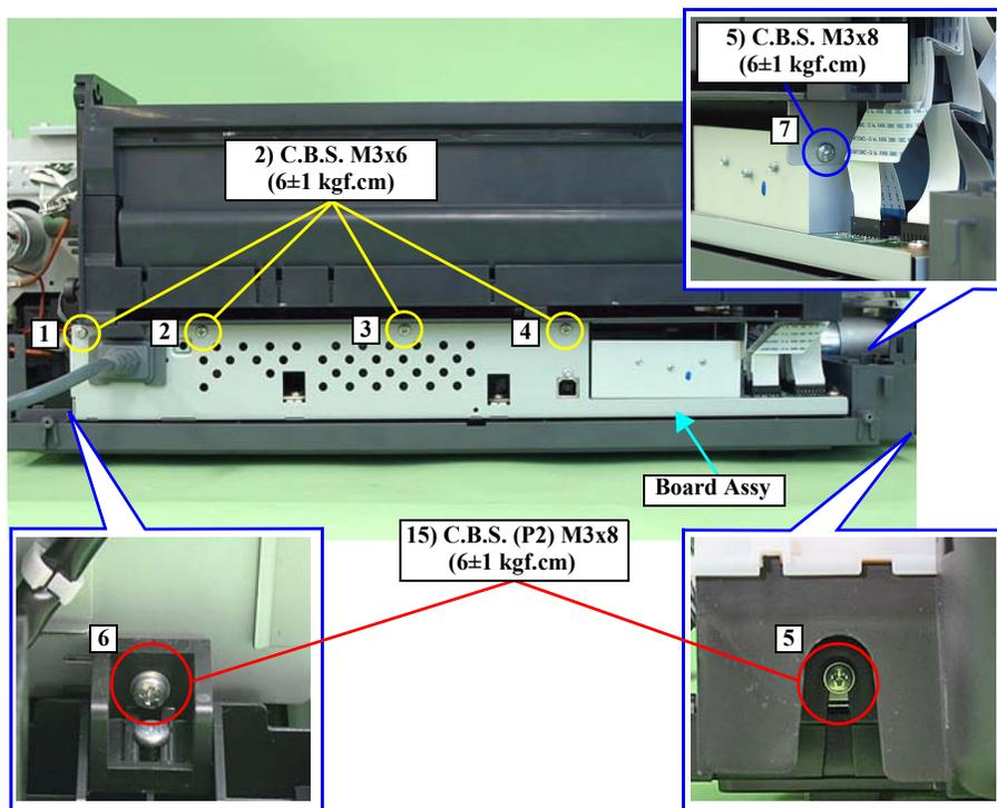
Figure 3-30. Removing the Board Assy (1)
