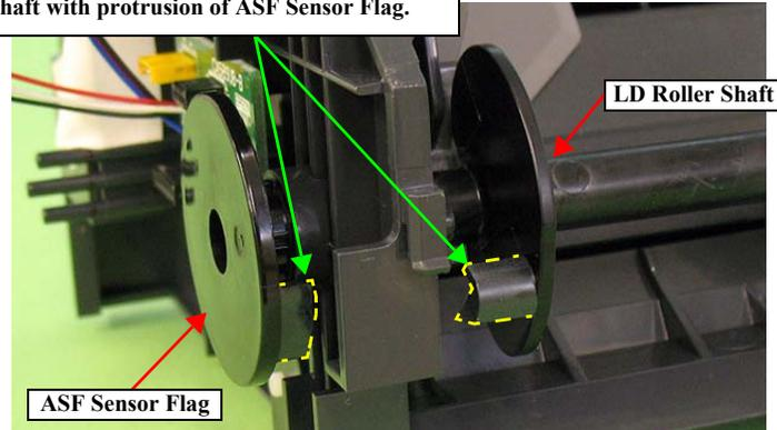
Figure 3-94. Reinstalling the ASF Sensor Flag
