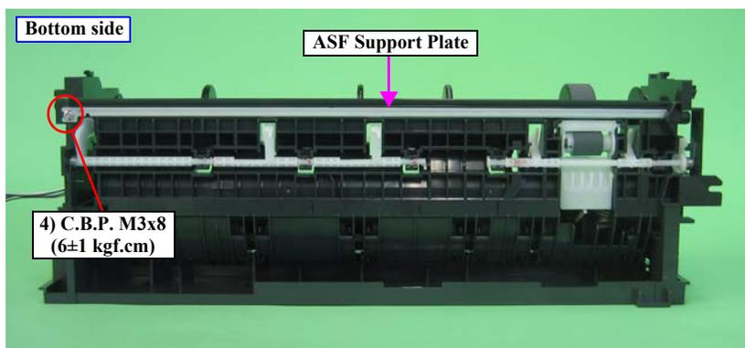
Figure 3-91. Removing the LD Roller (3)
