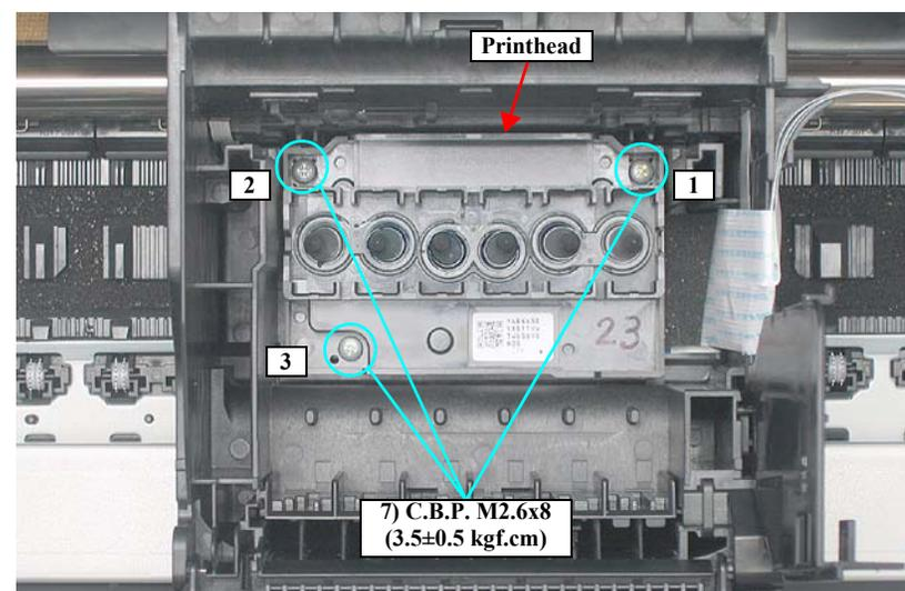
Figure 3-50. Removing the Printhead (1)
