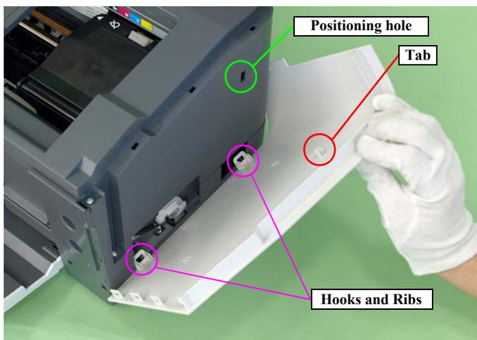
Figure 3-24. Reinstalling the Decoration Plate Left/Right
