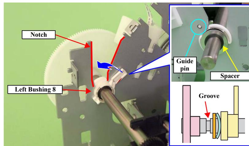
Figure 3-119. Removing the Spacer and Rotating the Left Bushing 8
