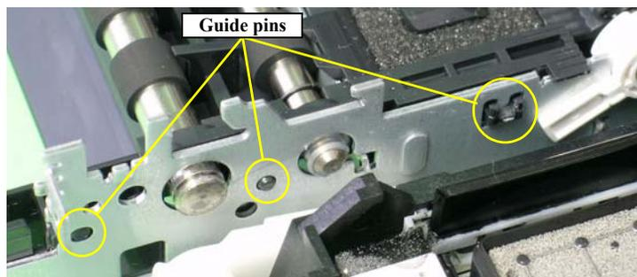
Figure 3-124. Reinstalling the Front Paper Guide
