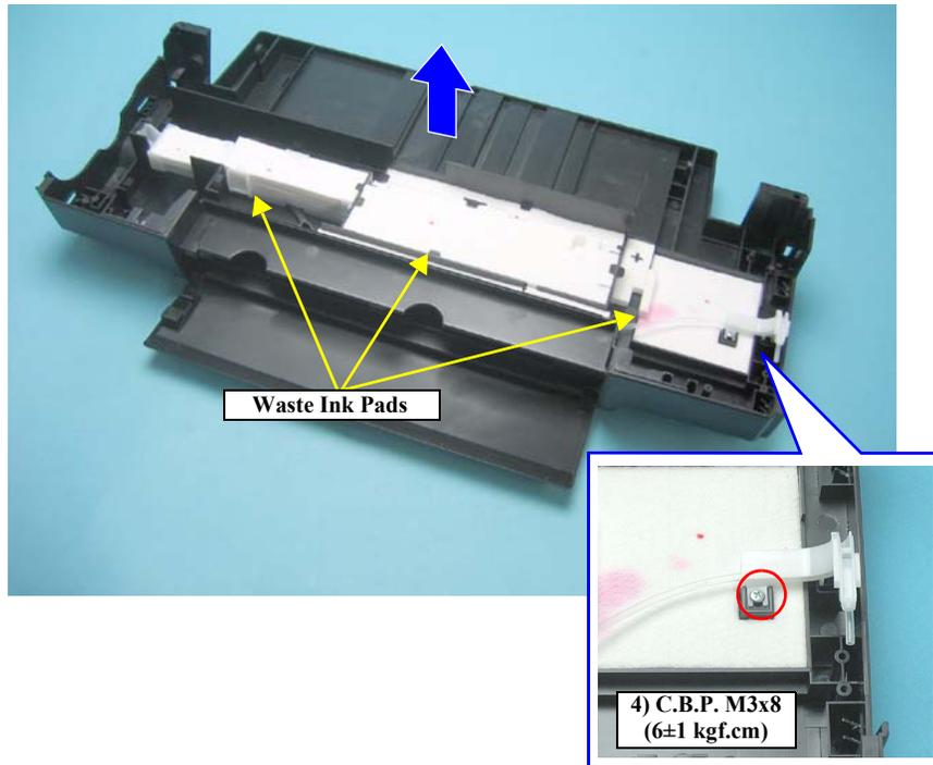
Figure 3-102. Removing the Waste Ink Pads
