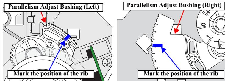
Figure 3-56. Marking Position
