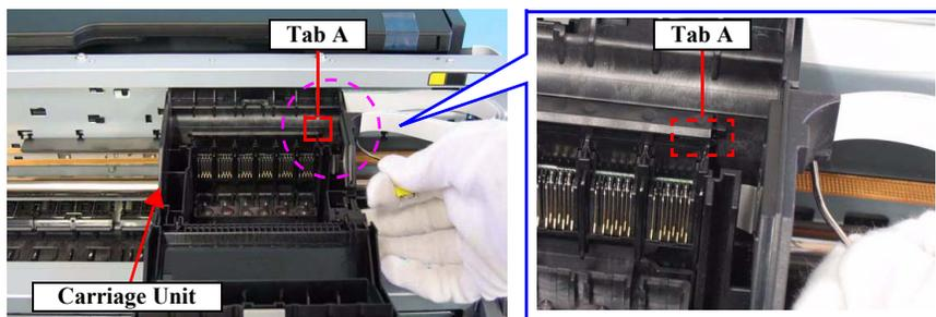
Figure 3-47. Removing the Adapter Guide Holder (2)
