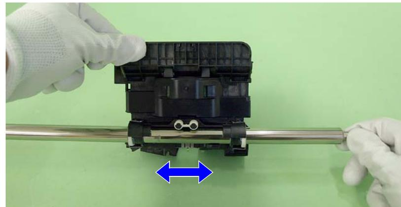
Figure 5-20. Lubricating the Carriage Shaft (2)
