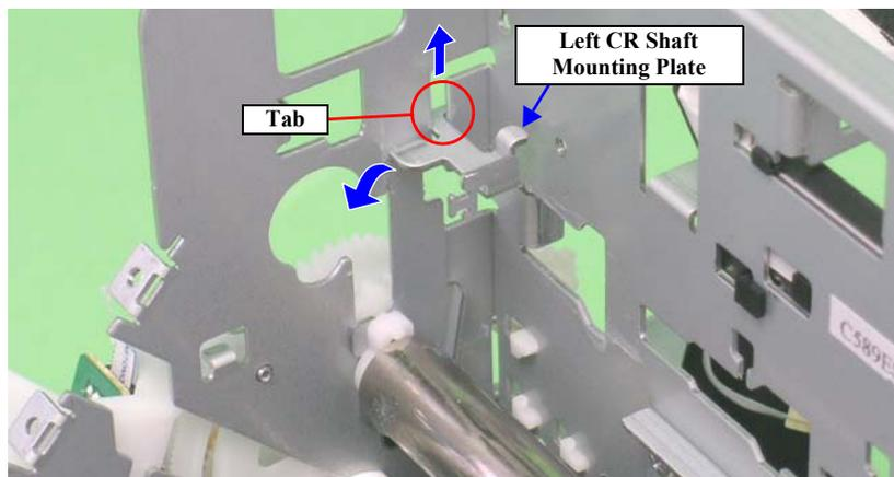
Figure 3-68. Rotating the Left CR Shaft Mounting Plate
