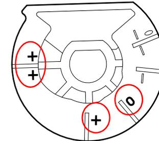
Figure 3-73. Right PG Cam Installation Direction
