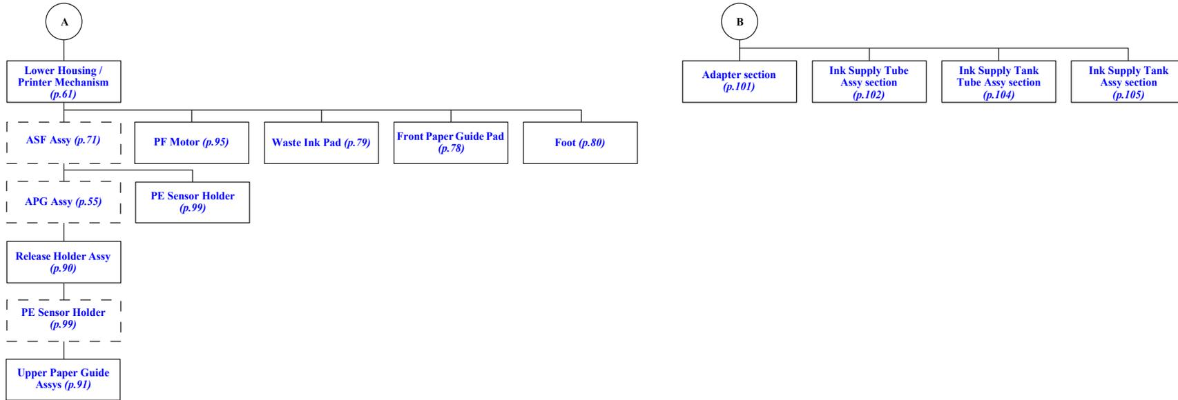
Figure 3-12. Disassembly Flowchart (2)
