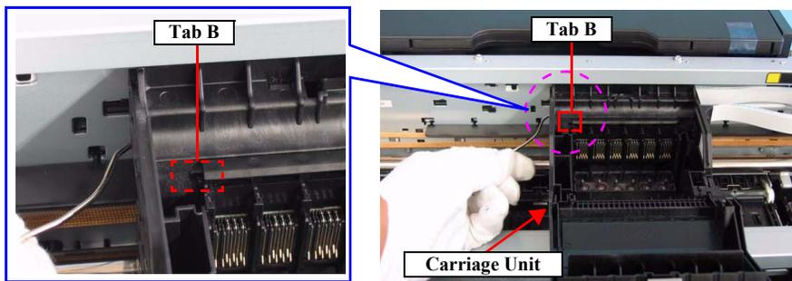
Figure 3-48. Removing the Adapter Guide Holder (3)
