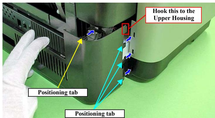
Figure 3-18. Reinstalling the Rear Housing
