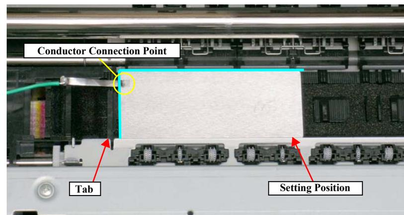
Figure 4-13. Setting the Adjustment Gauge
