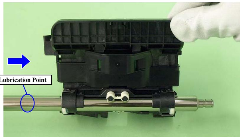
Figure 5-21. Lubricating the Carriage Shaft (3)
