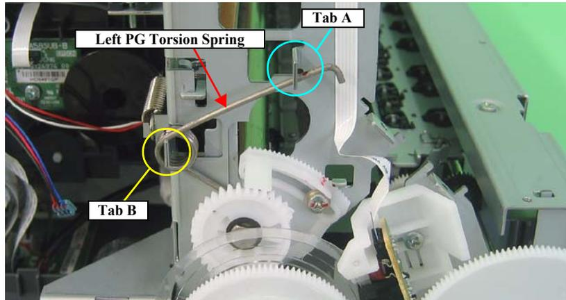
Figure 3-59. Removing the Left PG Torsion Spring
