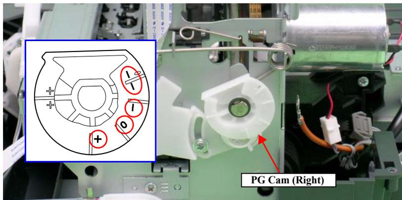
Figure 3-57. Adjusting the PG Cam
