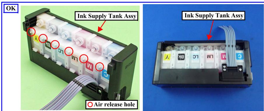
Figure 3-1. How to Place the Ink Tank Assy
