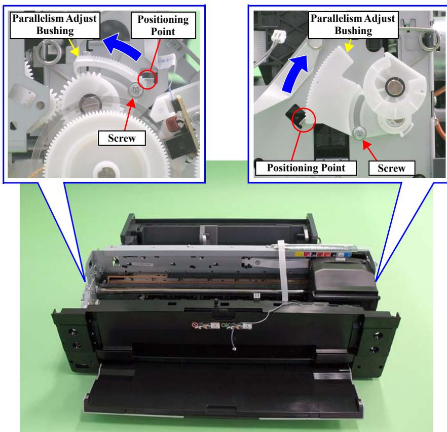
Figure 4-12. Setting the Parallelism Adjust Bushing
