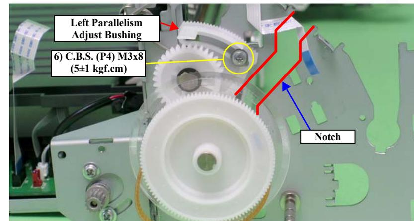
Figure 3-128. Rotating the Left Parallelism Adjust Bushing
