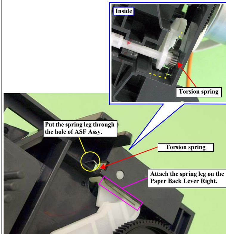
Figure 3-98. Reinstalling the Torsion Spring
