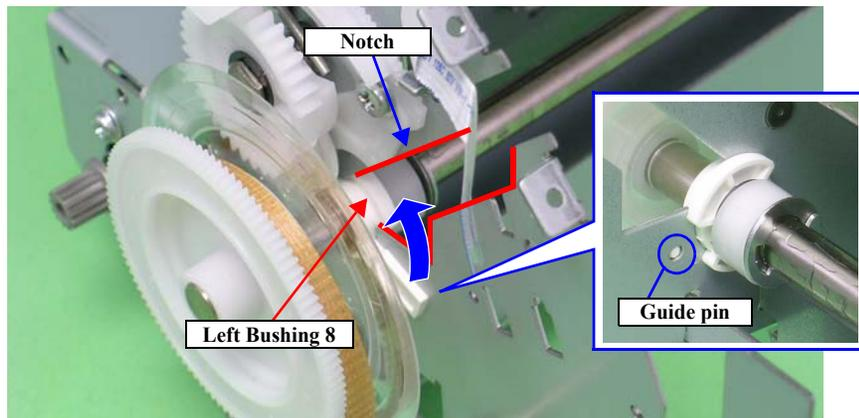
Figure 3-129. Rotating the Left Bushing 8
