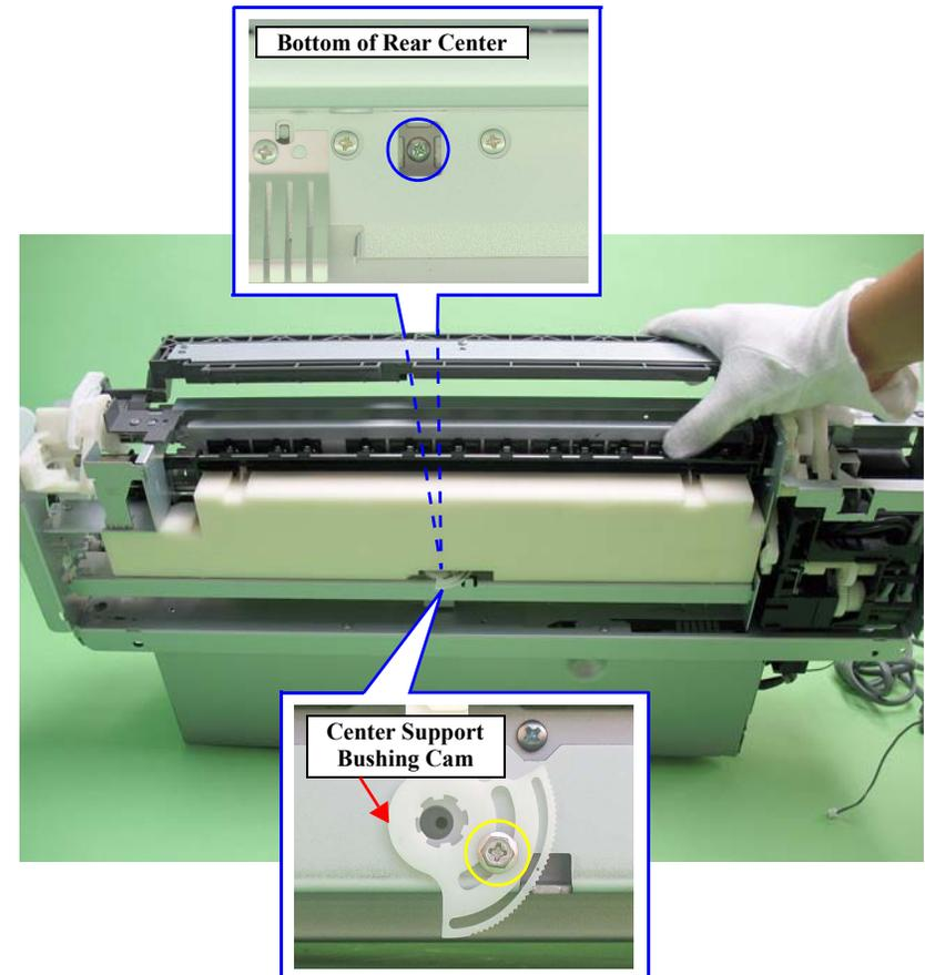
Figure 4-21. Center Support Bushing Cam and the Screw
