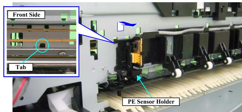
Figure 3-156. Removing the PE Sensor Holder
