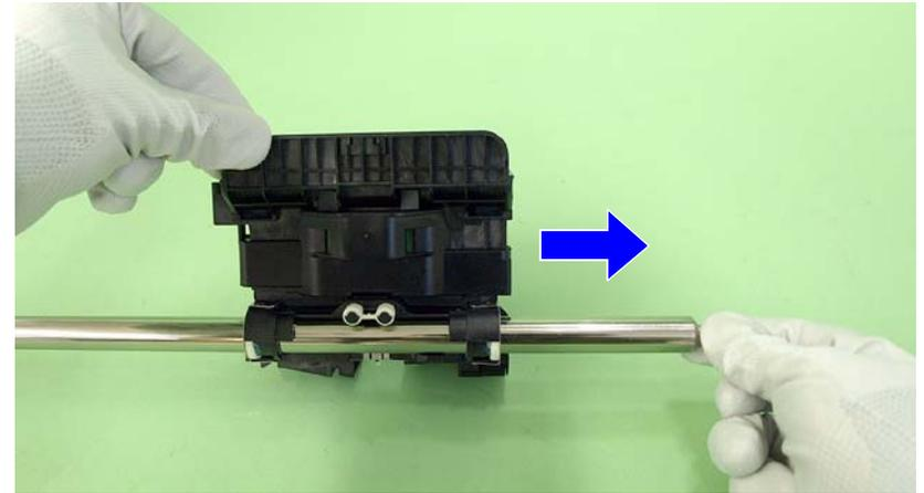
Figure 5-23. Lubricating the Carriage Shaft (5)
