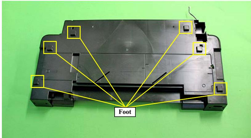
Figure 3-105. Removing the Foot
