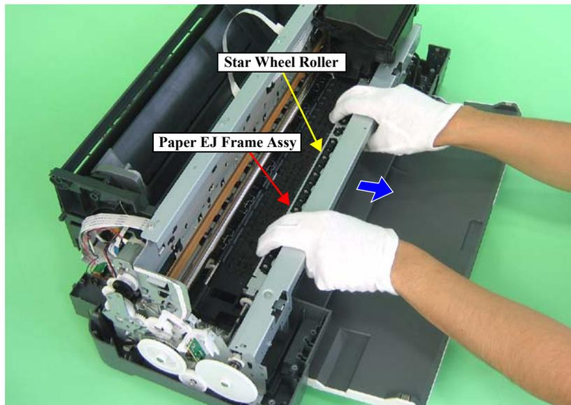
Figure 3-107. Removing the Paper EJ Frame Assy
