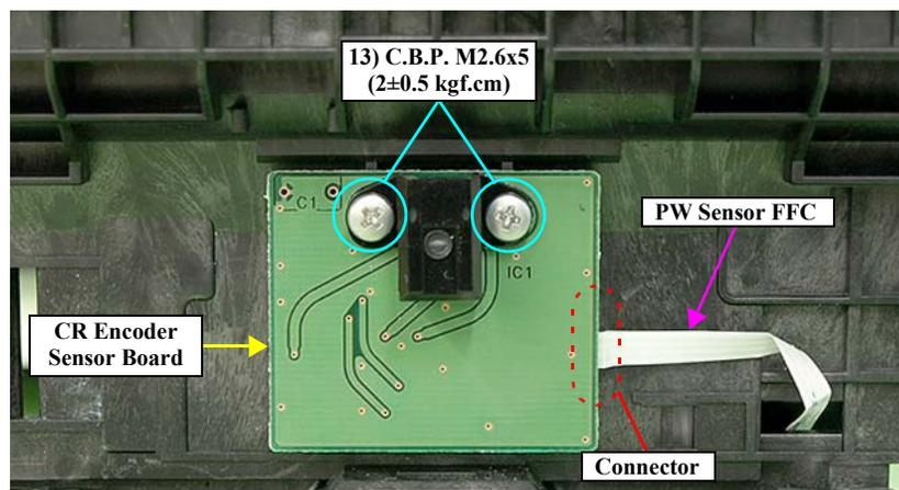
Figure 3-149. Removing the CR Encoder Sensor Board
