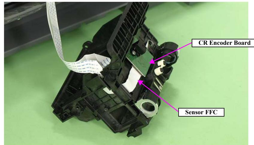
Figure 3-81. Removing the Carriage Unit
