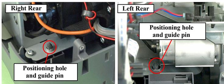
Figure 3-54. Reinstalling the Printer Mechanism
