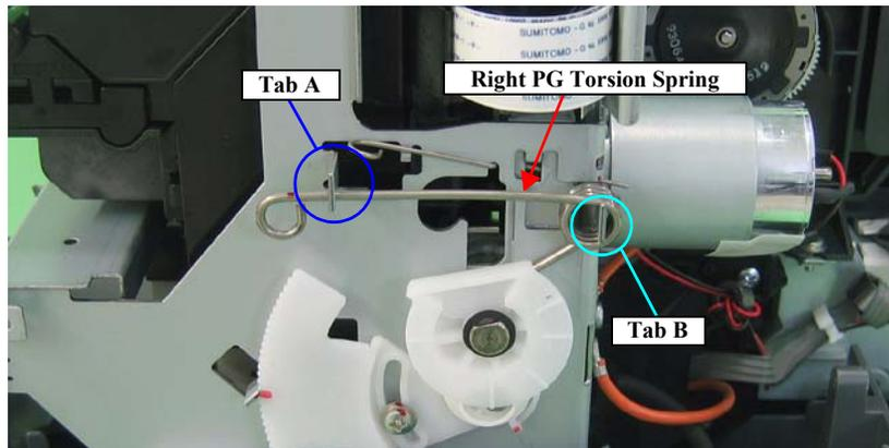
Figure 3-60. Removing the Right PG Torsion Spring
