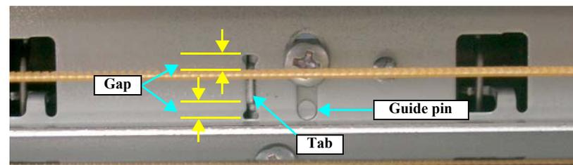
Figure 4-29. Checking the Position of Tab on the Guide Roller LD
