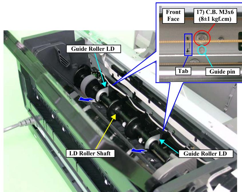
Figure 3-86. Removing the Guide Roller LD
