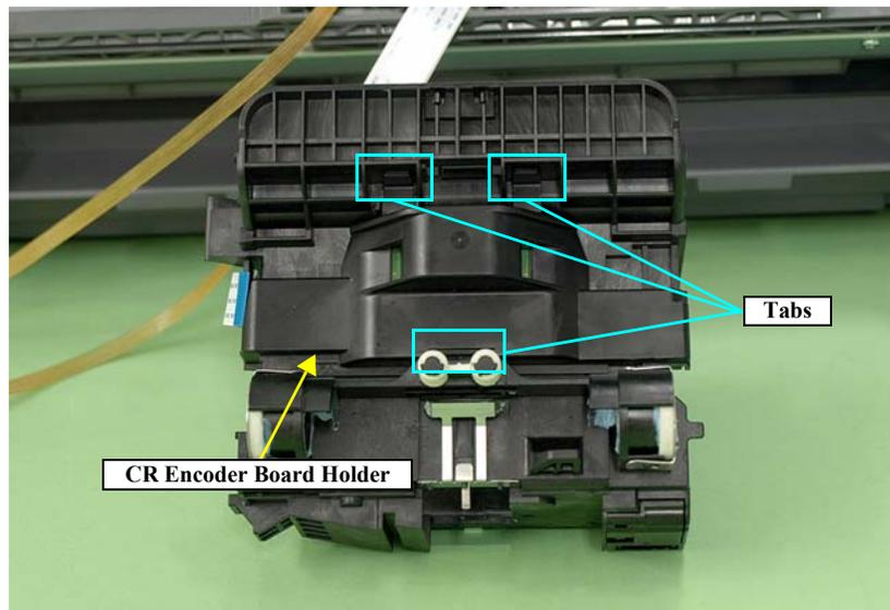
Figure 3-80. Removing the Belt Holder
