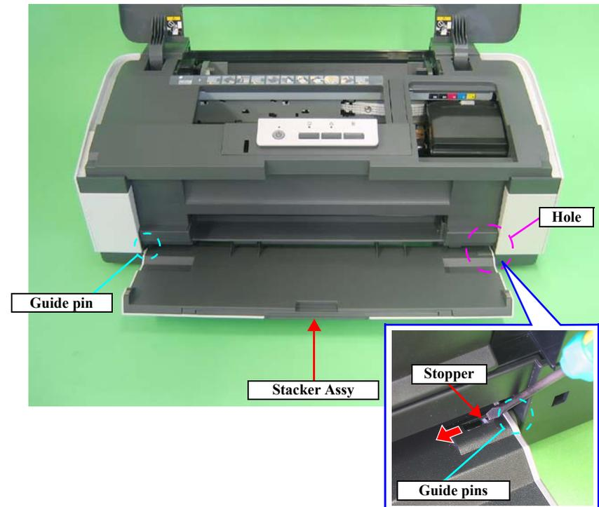
Figure 3-14. Removing Stacker Assy
