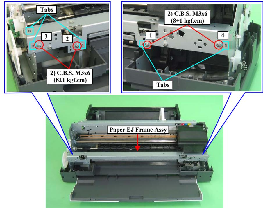
Figure 3-106. Screws that Secure the Paper EJ Frame Assy
