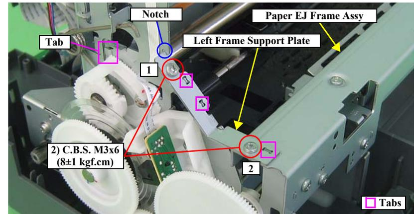
Figure 3-58. Removing the Left Frame Support Plate
