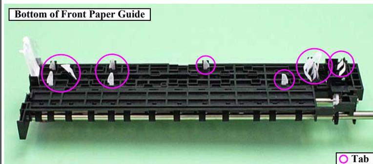
Figure 3-125. Checking the Front Paper Guide Pad
