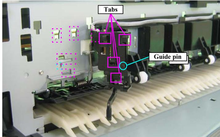
Figure 3-157. Reinstalling the PE Sensor
