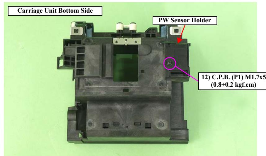
Figure 3-153. Removing the PW Sensor Holder
