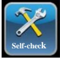
Press **Self check** enter secondary menu, choose test the function or sensor. On screen: carriage close, carriage open, cover clamp up, cover clamp down, Carriage right, carriage left, milling on/off, jogger on/off. Click the key and test if the part works normally. Press ↻ return to previous menu. (See right Pic)
