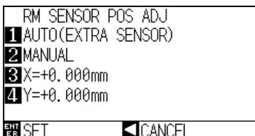
(16) Measure the offset between the printed cross mark and plotted cross mark.
