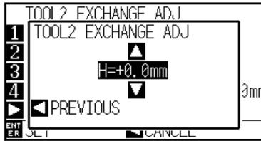
(16) Adjust the 2nd tool holder height by using the up or the down arrow key.
