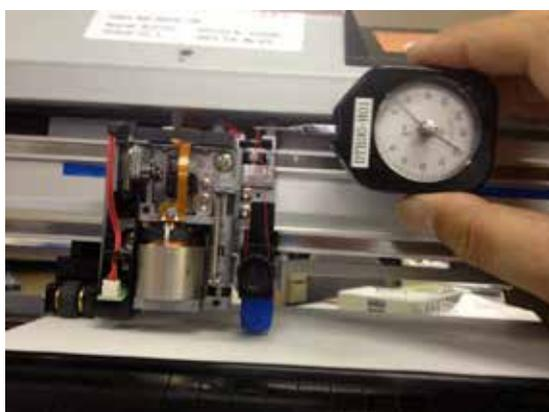
The measured pen force should be within the specification range ( $10 \pm 2$  g).
