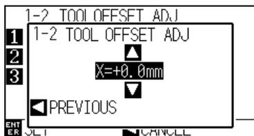
(16) Set the X-offset value. Press the UP ARROW key or DOWN ARROW key to change the number based on the pen 1 cross mark.
