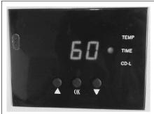
Press button after the temperature setting and the time light is ON. Press Up "△" or Down "▽" button to set time according to different transfer material.
