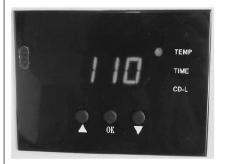
Press button, the temp light is ON. Press Up "△" or Down "▽" button to set temperature according to different transfer material.
