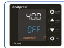
*Control panel P-4 is auto power-off setting with range 0-120min, 0 refers to not going enter into sleepy mode. As long as machine reaches to the set Temp. and is kept no in use for set time Say. 60mins, machine will enter into sleepy, display shows OFF and temperature cools down. You could touch any button on the control panel to wake up the machine.*
