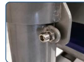
*After ten thousands of swing-away and press, maybe you need to adjust the position screw on the back column to make sure the upper heating platen and lower platen is always paralleled. (For Air Pro One and X)*
