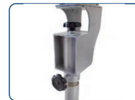
*There are two knob on the moveable caddy, upper knob is for caddy height adjustment (Max. 10cm), the lower knob is for anti-rotation, you can move around the upper machine when lower knob is in loosen status. (for Air Pro X only)*
