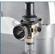
You could adjust the air pressure by air regulator, simply pull-up the black cap on its top, clockwise to increase, recommended pressure read-out 0.4-0.7Mpa.
