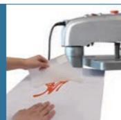
Take off the T-shirt and peel off the vinyl or paper depends on cold peel or hot peel.
