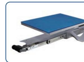
*It's ordinary if you feel some drag force when you slide out or slide back the lower platen, as Magnetic Tech is applied, which makes sure lower platen won't slide back when you are threading a T-shirt, also makes sure upper & lower platens are in correct location after you slide the drawer back. (For Air Pro One and X)*
