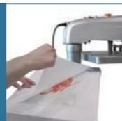
Position the substrate and preheat to remove the wrinkles or moisture, continue to place the graphics design on paper or vinyl on substrate and cover with a Teflon sheet.
