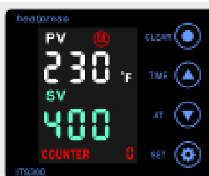
User can wake up heat press and start heating by touching any key
