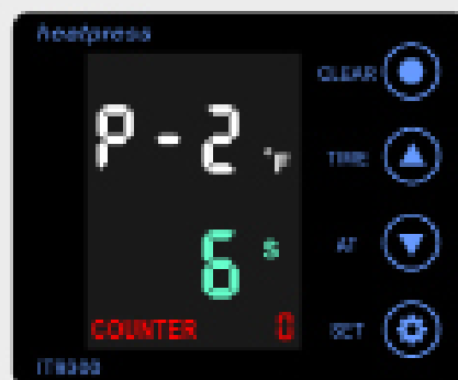
P-2: Time Setting Mode. Touch SET & ▲▼ keys to set desired time
