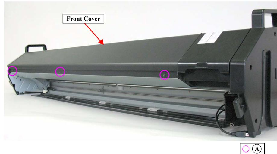
Figure 4-200. Removing the Front Cover (1)
